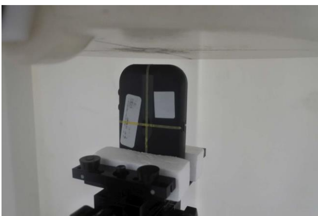
Right Side, Test Separation 10 mm
