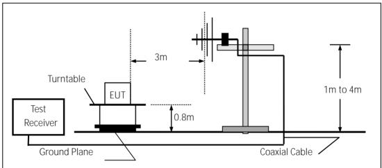
(c) For radiated emissions above 1000MHz
