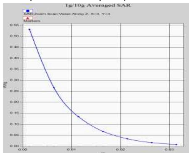
Z-Scan at power reference point (LTE Band38 ANT13)
