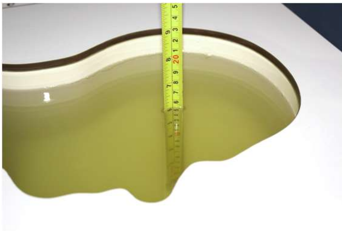
Picture 7-7 Liquid depth in the Head Phantom (3300-3900 MHz)
