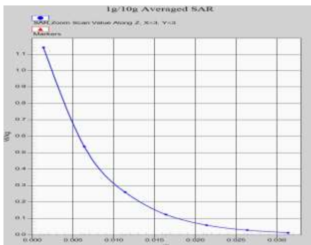
Z-Scan at power reference point (N41 ANT13)
