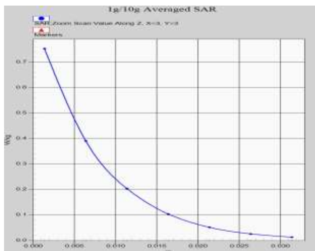
Z-Scan at power reference point (N7 ANT13)
