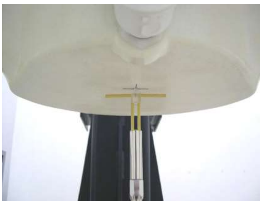
Picture 8.2 Photo of Dipole Setup
