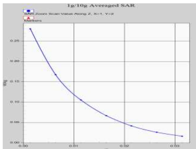
Z-Scan at power reference point (GSM1900 ANT31)
