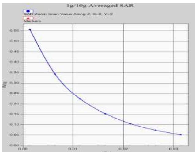
Z-Scan at power reference point (GSM850 ANT41)
