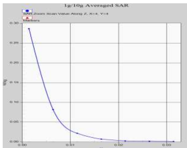
Z-Scan at power reference point (N78 ANT12)
