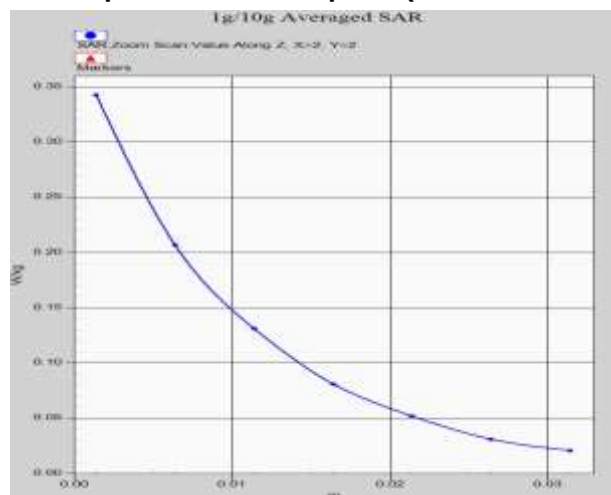
Z-Scan at power reference point (LTE Band2 ANT31)
