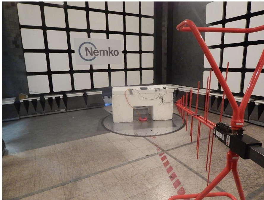
Figure 7.2-9: Radiated spurious emissions – below 1 GHz
