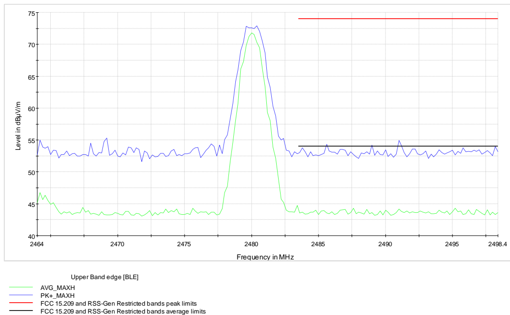
Figure 7.2-4: Radiated spurious emissions on upper band edge [BLE]
