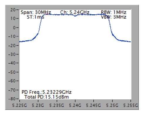
Power Density Plot on Configuration IEEE 802.11ac MCS0/Nss1 VHT40 / Chain 1 + Chain 2 + Chain 3 + Chain 4 / 5230 MHz
