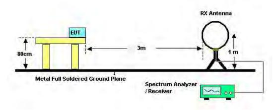
For Radiated Emissions: 30MHz~1GHz
