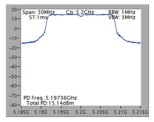
Power Density Plot on Configuration IEEE 802.11ac MCS0/Nss1 VHT20 / Chain 1 + Chain 2 + Chain 3 + Chain 4 / 5240 MHz
