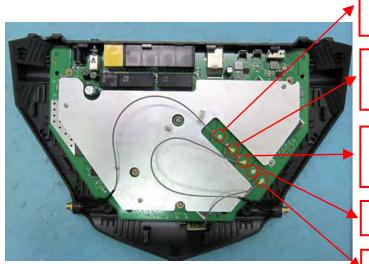
2.4GHz: Chain 1 / Connect to Ant 15GHz: Chain 4 / Connect to Ant 1
