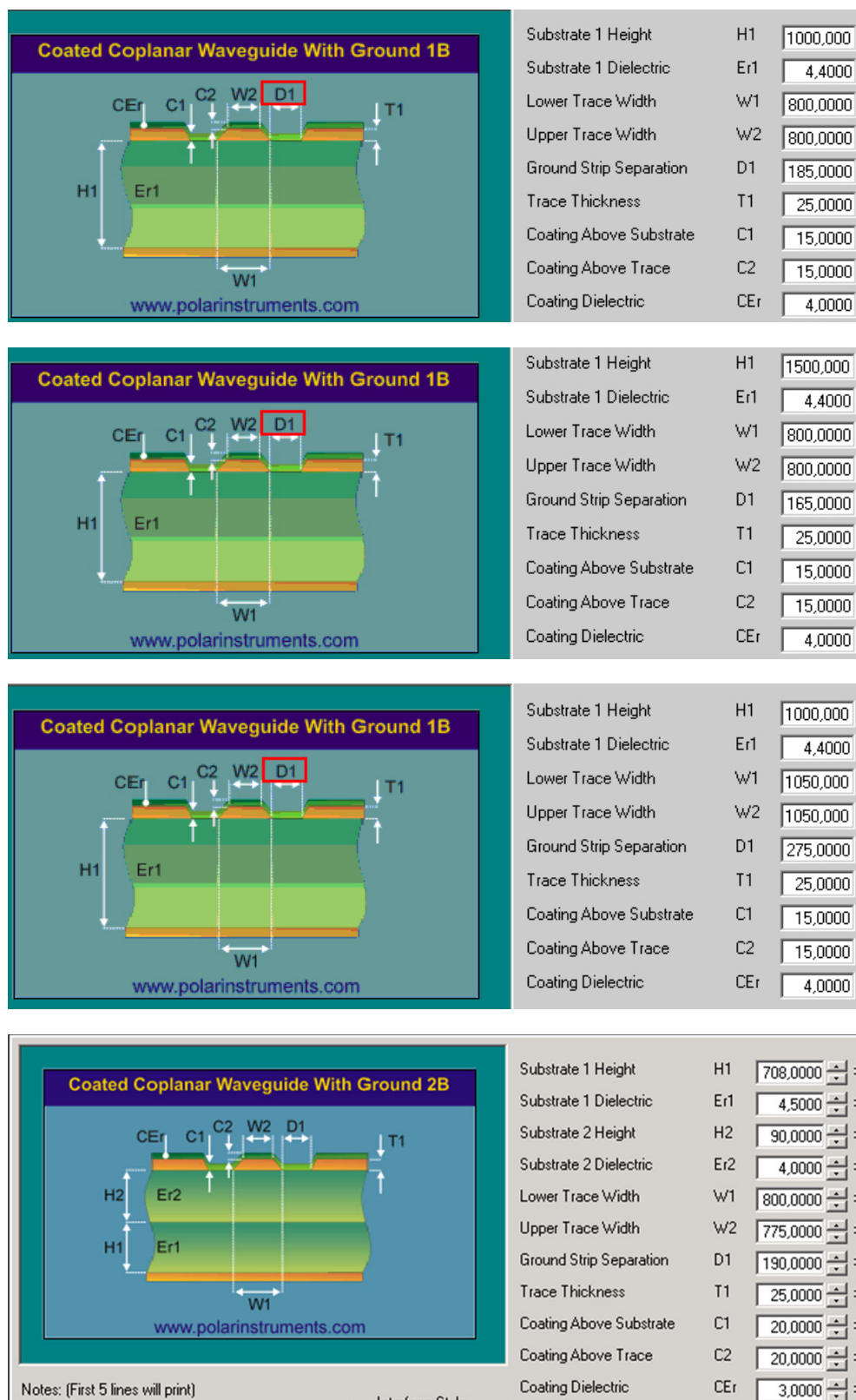
Figure 8: Micro-Stripline line arrangement samples
