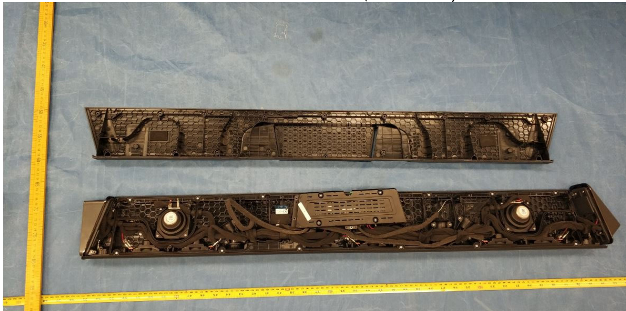
Internal View of EUT-2 (sound bar)
