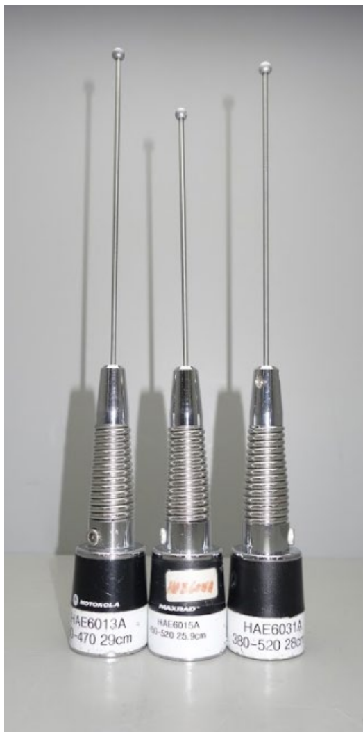
UHF1 Antenna kit numbers, from left to right HAE6013A, HAE6015A, HAE6031A
