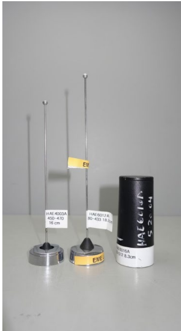
UHF1 Antenna kit numbers, from left to right HAE4003A, HAE6012A, HAE6016A
