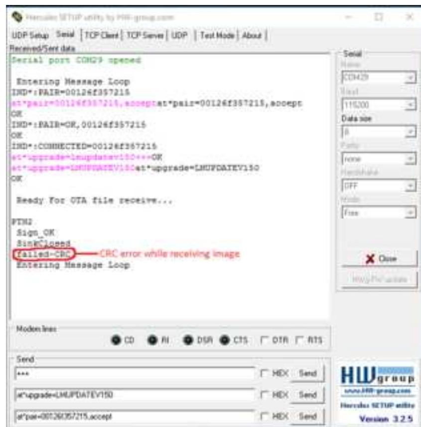
Figure 4: UART messages when the CRC of the received image does not match
