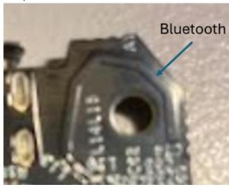
Antenna description: Monopole Connector type: PCB trace
