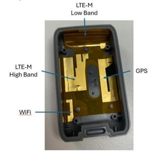
Antenna description: Monopole Connector type: PCB trace
