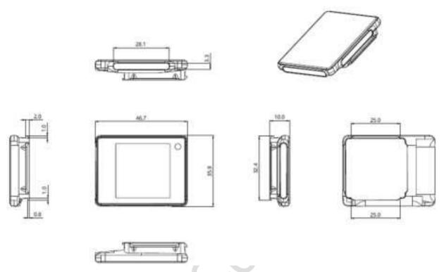
Figure 2-3 Mechanical drawing for 1.54"
