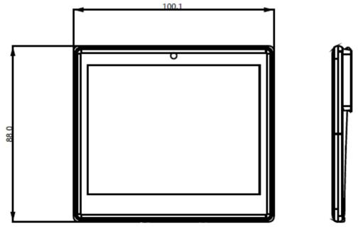
Figure 2-8 Mechanical drawing for 4.2"
