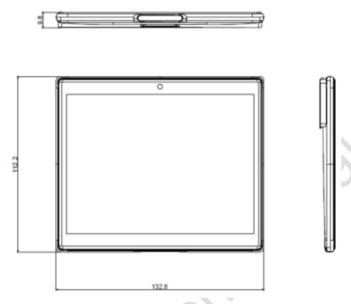
Figure 2-9 Mechanical drawing for 5.83"
