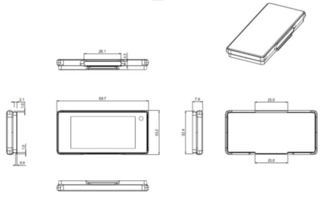
Figure 2-4 Mechanical drawing for 2.13"
