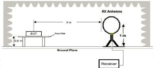
2. Radiated Emission Test-Up Frequency 30MHz~1GHz
