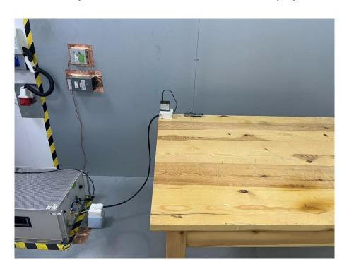
Set-up for Radiated Emission (RE), Below 1GHz
