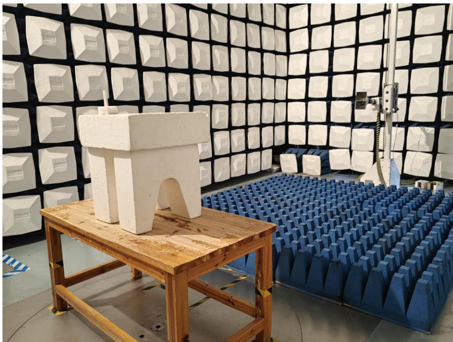
Test Setup For Radiated Emission (Above 1GHz)
