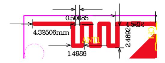
**Antenna Type: PCB Antenna**
