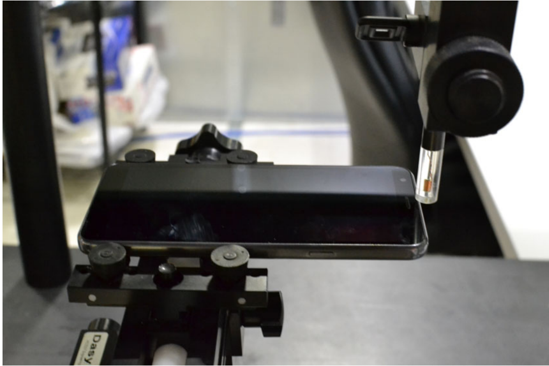
Figure 16-1 Test Setup for Wireless Device
