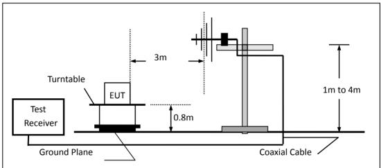
(c) For radiated emissions above 1000MHz
