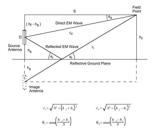
Figure 1. UT MPE Calculation Geometry
