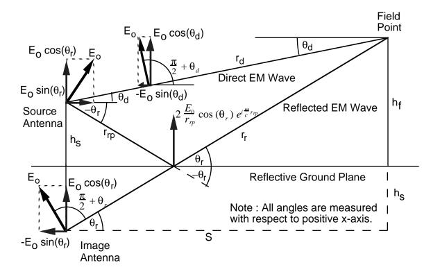
Distance to Ground Plane Reflection Point  $r_{rp} = h_s \csc(\theta_r)$
