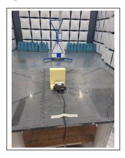
Radiated Spurious Emissions: Greater Than 1 GHz
