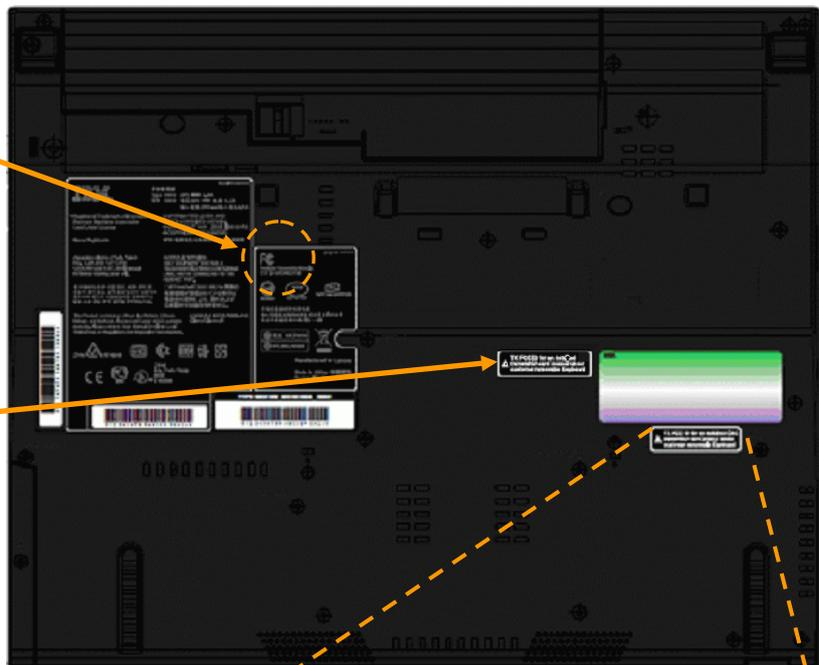
TX FCC ID for an installed transmitter card located under customer removable Keyboard
