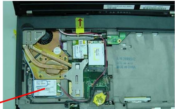
The certification label is stuck on the topside of the applying transmitter device, and the FCC ID is visible when the keyboard assembly is removed.
