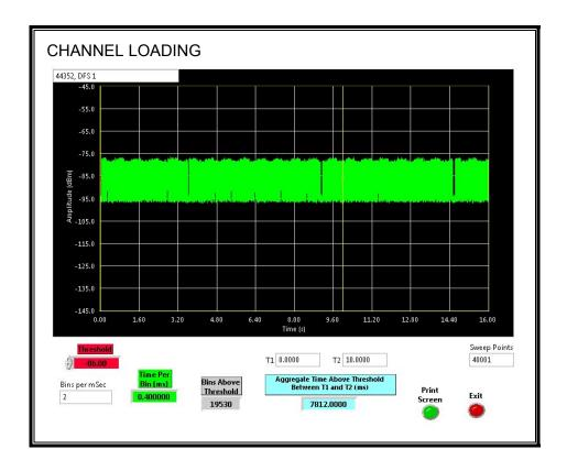
The level of traffic loading on the channel by the EUT is 78.12%
