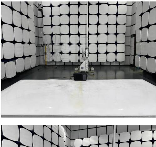
1.1. Photo of Radiated Emission test
