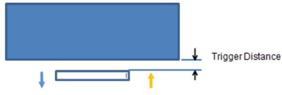
Picture: Proximity sensor triggering distances assessment Front Side and Back side
