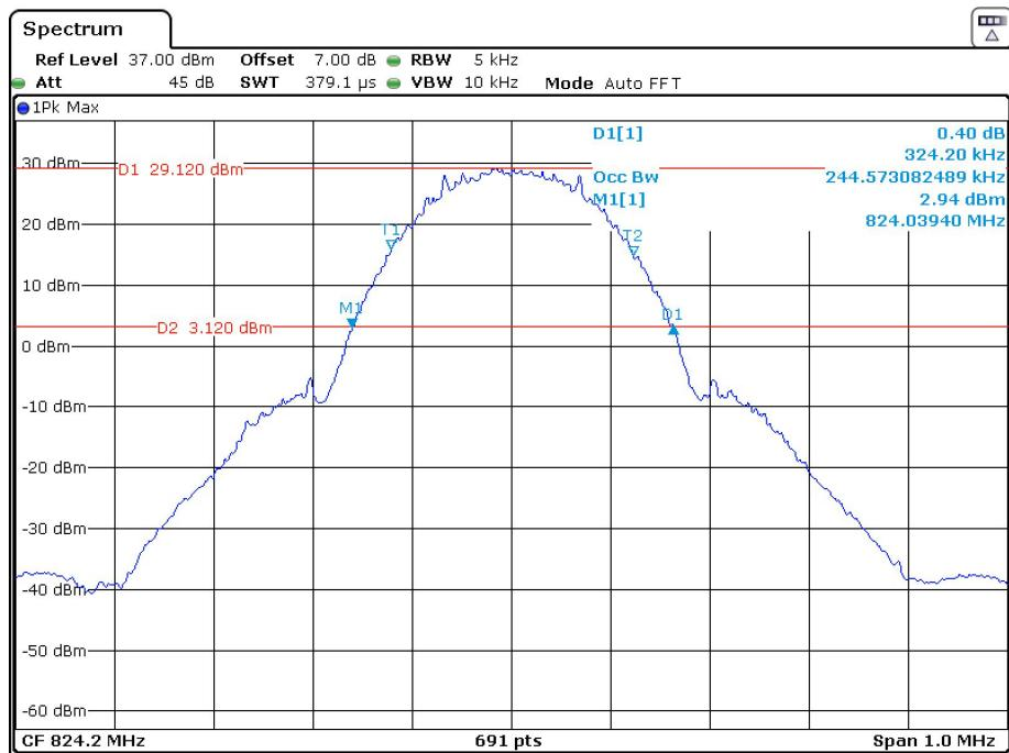
**26 dB Emissions &99% Occupied Bandwidth for GSM(GMSK) Mode, Middle channel**
