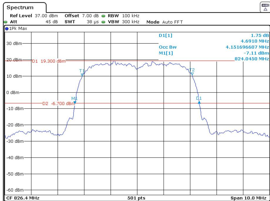
**26 dB Emissions & 99% Occupied Bandwidth for RMC (BPSK) Mode, Middle channel**
