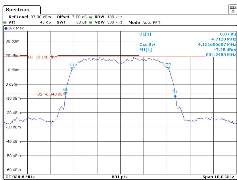
**26 dB Emissions &99% Occupied Bandwidth for RMC (BPSK) Mode, High channel**
