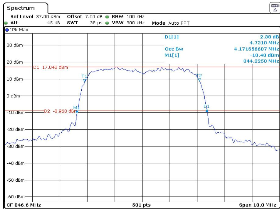
**PCS Band (Part 24E)****26 dB Emissions & 99% Occupied Bandwidth for GSM (GMSK) Mode, Low channel**
