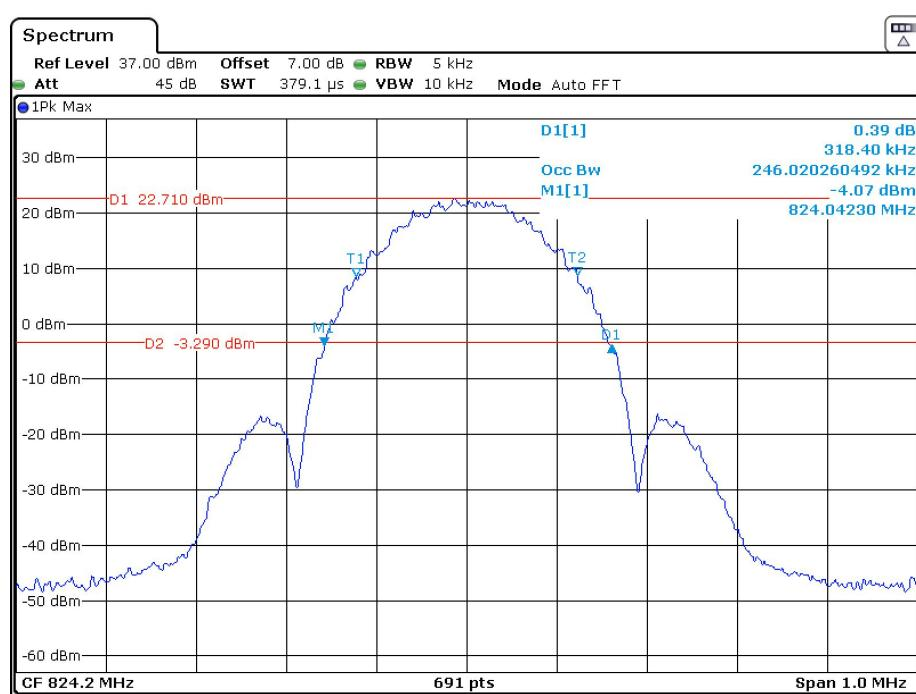
**26 dB Emissions &99% Occupied Bandwidth for EDGE Mode, Middle channel**
