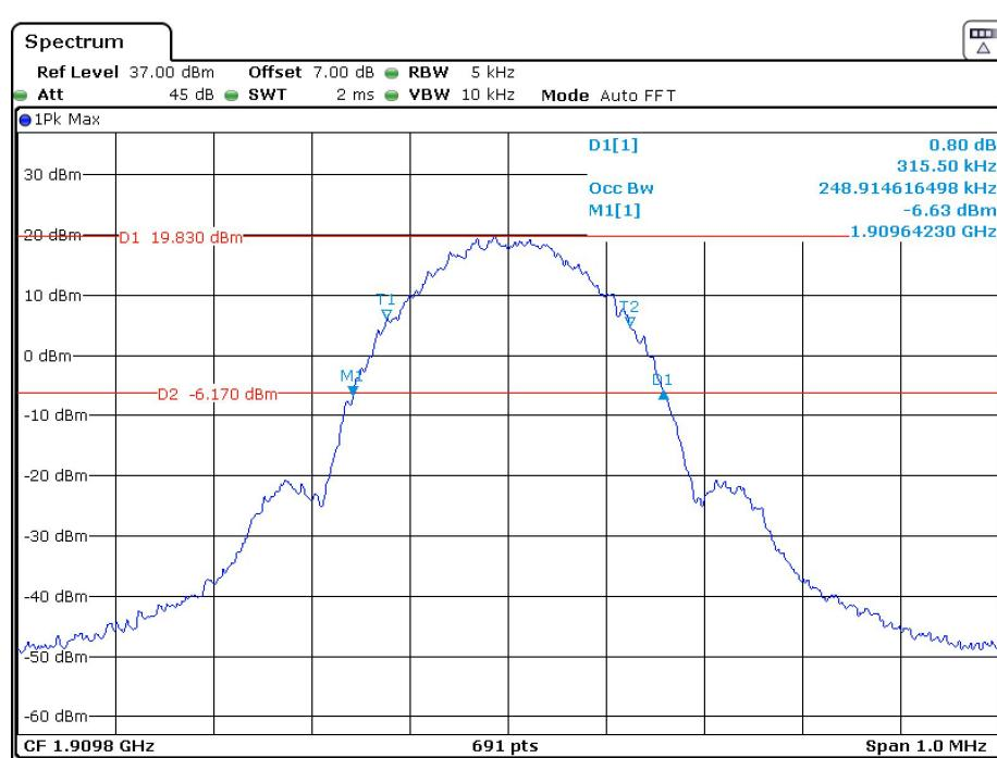
**26 dB Emissions &99% Occupied Bandwidth for RMC (BPSK) Mode, Low channel**
