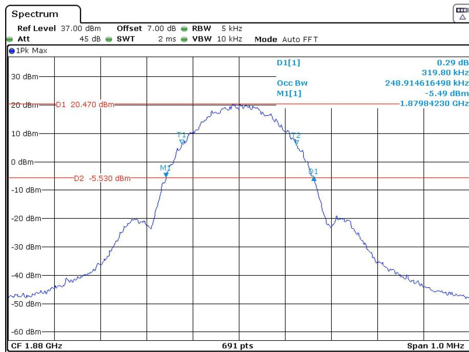
**26 dB Emissions &99% Occupied Bandwidth for EDGE Mode, High channel**
