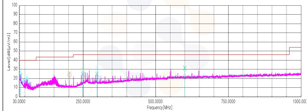
**[PoE 48 V]****Test results for fundamental****15.225 (a) 13.553-13.567 MHz****[Face-on]**
