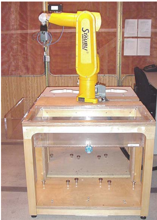
DASY4 SAR Measurement System with validation phantom
