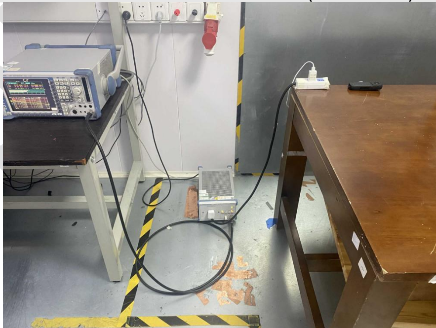
Conducted Emissions at Mains Terminals (150kHz-30MHz)
