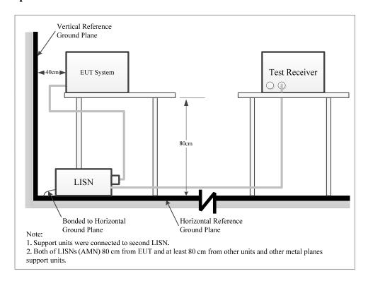
The setup of EUT is according with per ANSI C63.4-2014 measurement procedure. The specification used was with the FCC Part 15 B Class B limits.
