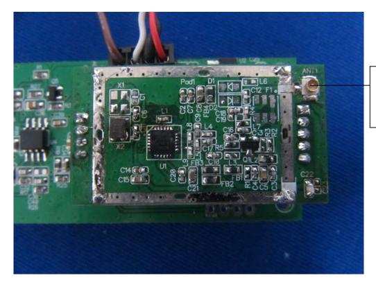
Microphone Antenna ipex connector
