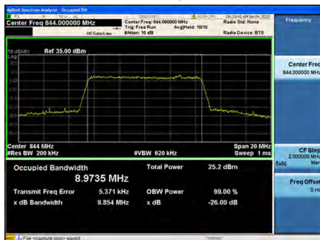
Band5 / 10MHz / High CH / 16QAM
