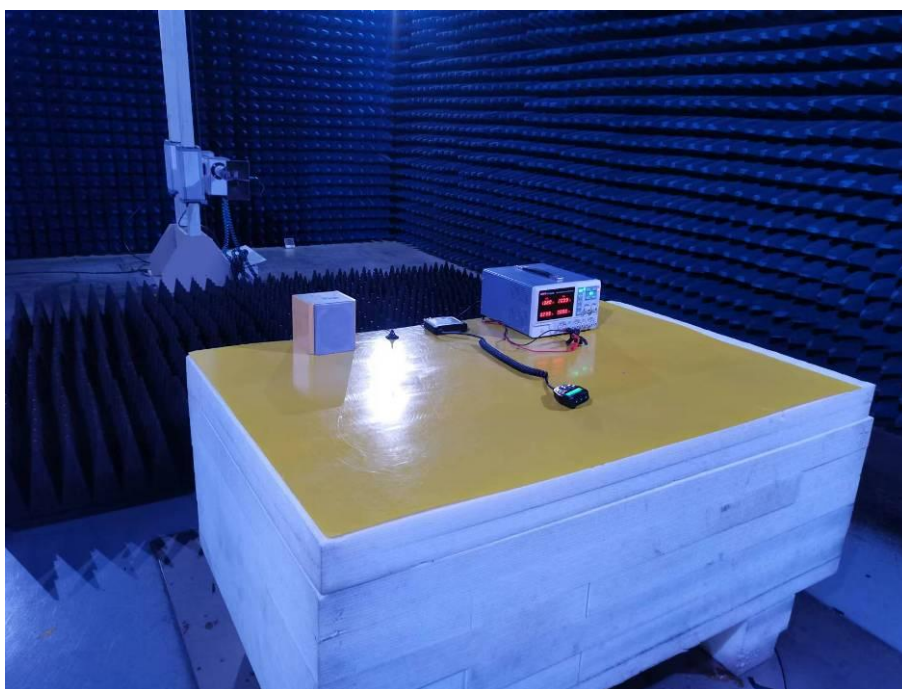
Photo of Radiated Emission Measurement (Above 1G)
