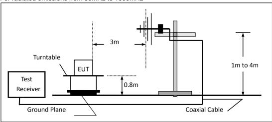
(c) For radiated emissions above 1000MHz
