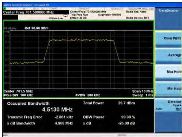
LTE Band 12 16QAM 5MHz CH-Middle
