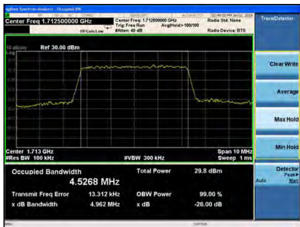
LTE Band 4 QPSK 5MHz CH-Middle
