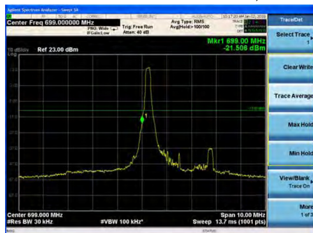
LTE Band 12 16QAM 3MHz CH-Low, 100%RB
