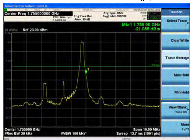
LTE Band 4 QPSK 3MHz CH-High, 1 RB
