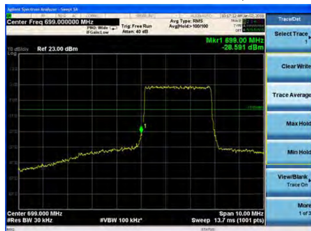
LTE Band 12 16QAM 3MHz CH-Low, 100%RB
