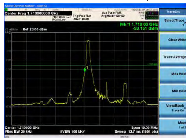
LTE Band 4 QPSK 3MHz CH-Low, 1 RB
