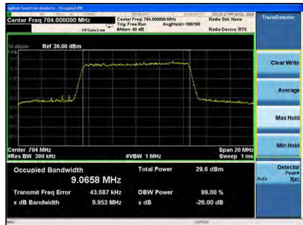
LTE Band 12 16QAM 10MHz CH-Middle
