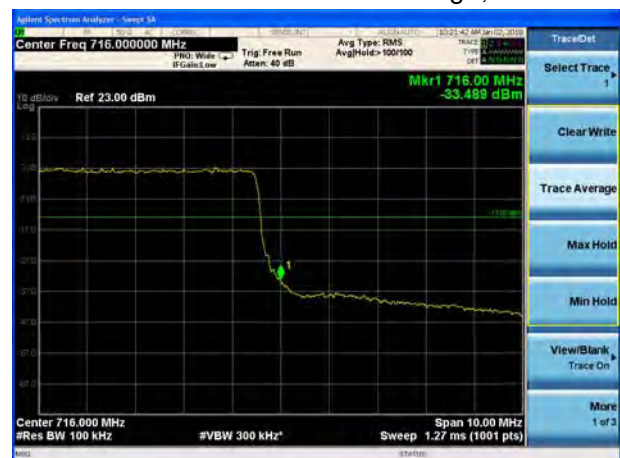
LTE Band 12 QPSK 10MHz CH-High, 100%RB
