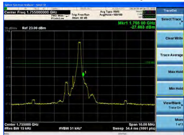
LTE Band 4 QPSK 1.4MHz CH-High, 100%RB
