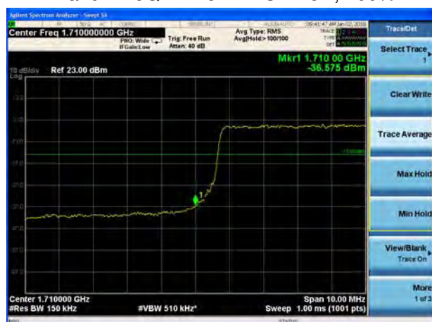
LTE Band 4 16QAM 20MHz CH-Low, 1 RB
