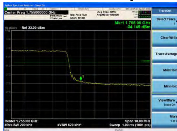
LTE Band 4 16QAM 20MHz CH-High, 100%RB
