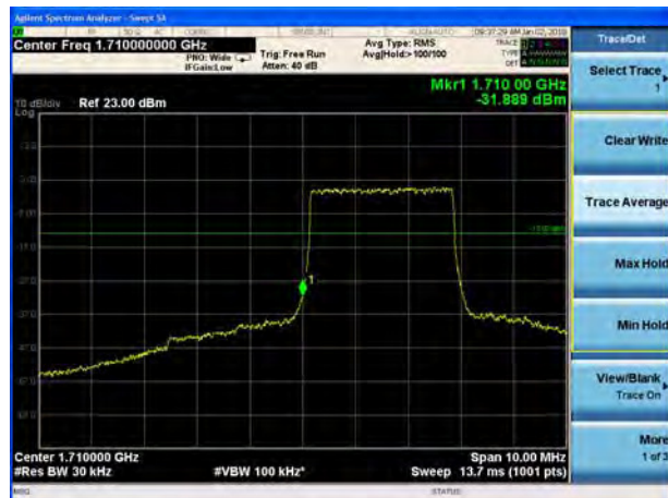
LTE Band 4 16QAM 5MHz CH-Low, 1 RB
