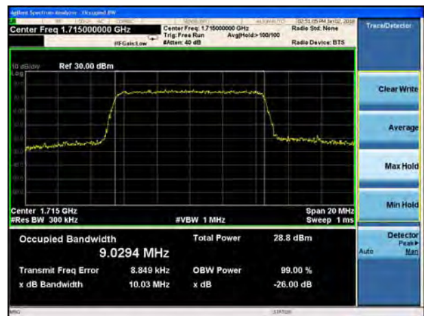
LTE Band 4 QPSK 10MHz CH-Middle
