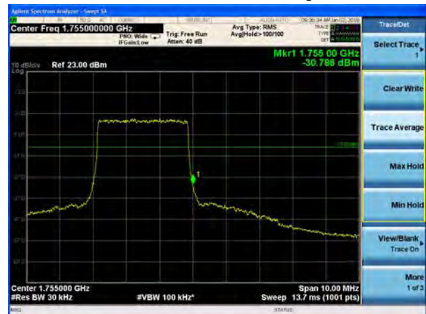
LTE Band 4 16QAM 5MHz CH-High, 1 RB
