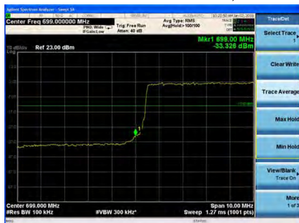
LTE Band 12 QPSK 10MHz CH-Low, 100%RB
