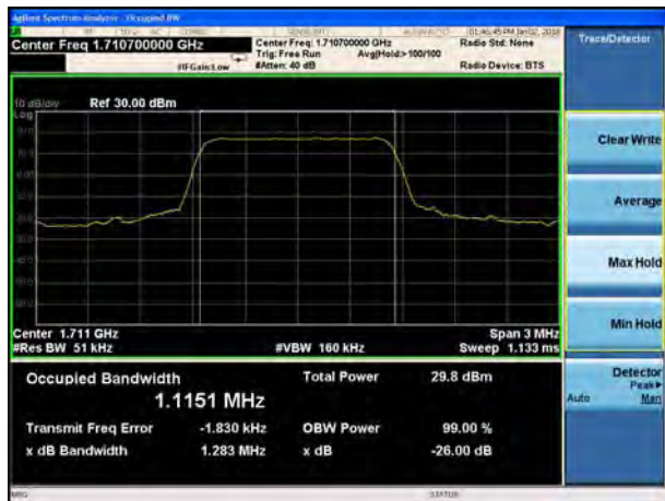
LTE Band 4 QPSK 1.4MHz CH-Middle
