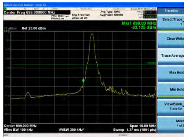
LTE Band 12 QPSK 10MHz CH-Low, 100%RB
