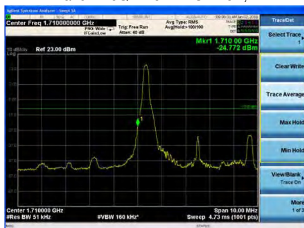
LTE Band 4 16QAM 5MHz CH-Low, 100%RB
