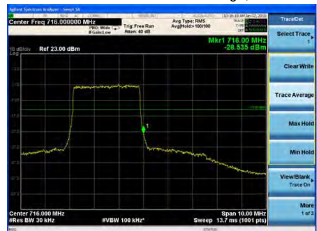
LTE Band 12 16QAM 3MHz CH-High, 100%RB
