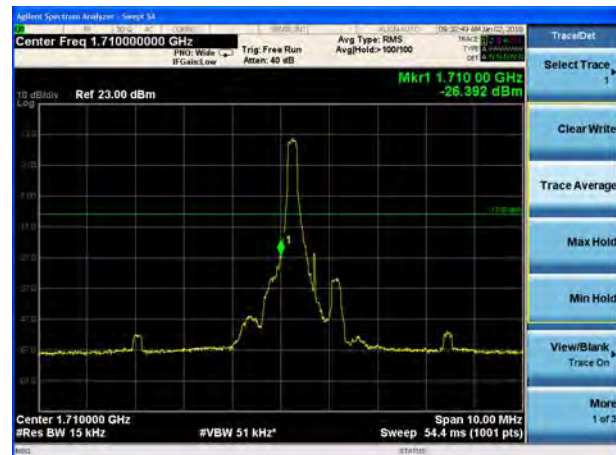
LTE Band 4 QPSK 1.4MHz CH-Low, 100%RB
