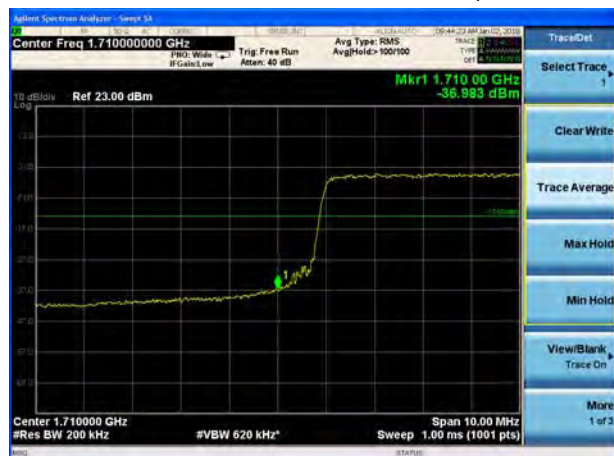
LTE Band 4 16QAM 20MHz CH-Low, 100%RB
