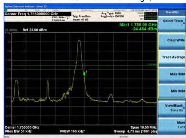
LTE Band 4 16QAM 5MHz CH-High, 100%RB
