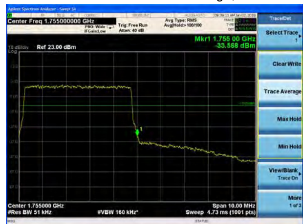
LTE Band 4 16QAM 5MHz CH-High, 100%RB
