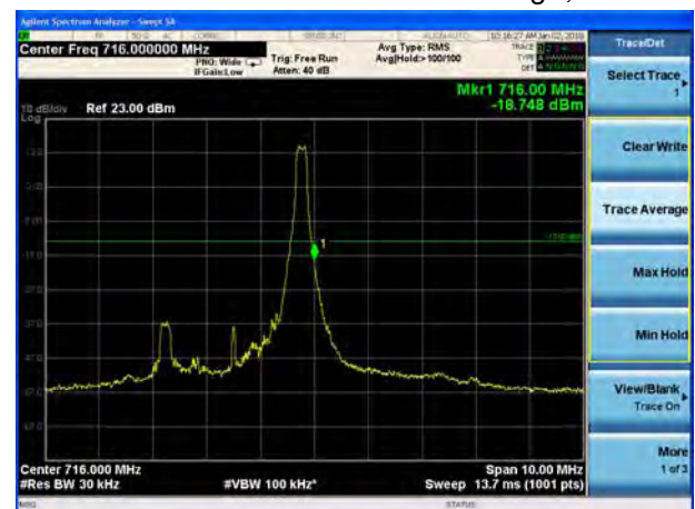
LTE Band 12 16QAM 3MHz CH-High, 100%RB
