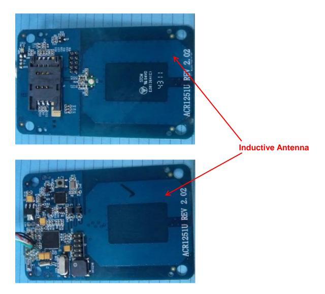
Note: The EUT has a printed antenna on PCB. which was permanently attached, the antenna gain is 0 dBi .
