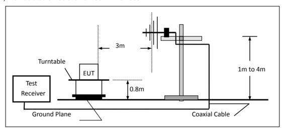
(c) For radiated emissions above 1000MHz
