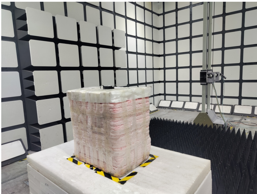
Radiated Emissions View (1-18 GHz)
