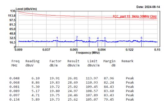
Project No.: XMDN240311-12032E-RF Test Mode: Transmitting(Perpendicular) EUT Model: A08S Test distance: 3m Temp/Humi/ATM: 24.2<sup>°</sup>C/59%/100.1kPa Tested by: Wlif Wu Power Source: DC 12V from adapter
