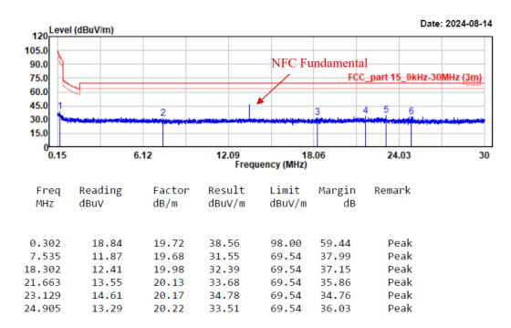
Project No.: XMDN240311-12032E-RF Test Mode: Transmitting(Perpendicular) EUT Model: A08S Test distance: 3m Temp/Humi/ATM: 24.2°C/59%/100.1kPa
