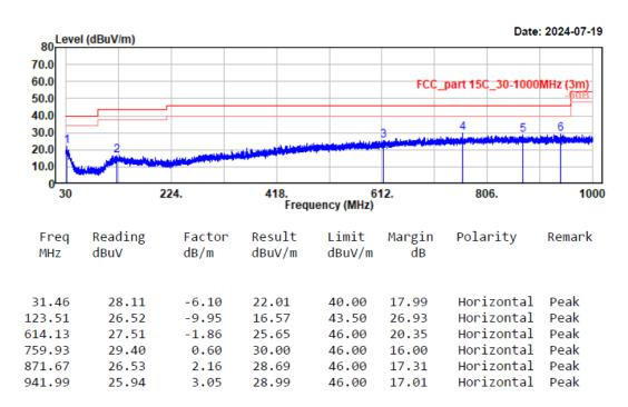
Project No.: XMDN240311-12032E-RF Test Mode: Transmission(NFC) EUT Model: A08S Test distance: 3m Temp/Humi/ATM: 23.5°C/55%/100.1kPa Tested by: Wlif Wu Power Source: DC 12V from adapter
