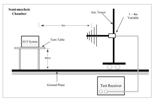
The radiated emission tests were performed in the 3-meter chamber a test site, using the setup accordance with the ANSI C63.10-2020. The specification used was the FCC Part Subpart C limits.
