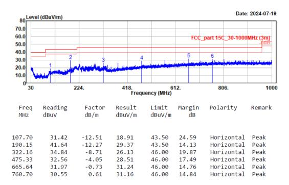
Project No.: XMDN240311-12032E-RF Test Mode: Transmission(NFC) EUT Model: A08S Test distance: 3m Temp/Humi/ATM: 23.5℃/55%/100.1kPa Tested by: Wlif Wu Power Source: DC 48V from PoE
