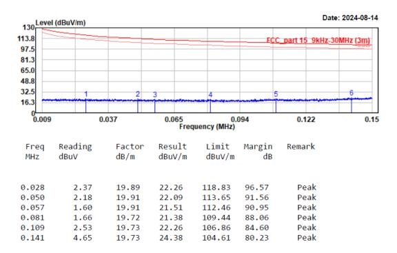
Project No.: XMDN240311-12032E-RF Test Mode: Transmitting(Ground-parallel) EUT Model: A08S Test distance: 3m Temp/Humi/ATM: 24.2<sup>°</sup>C/59%/100.1kPa Tested by: Wlif Wu Power Source: DC 12V from adapter
