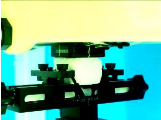
Rear Face of EUT with 0 mm Gap
