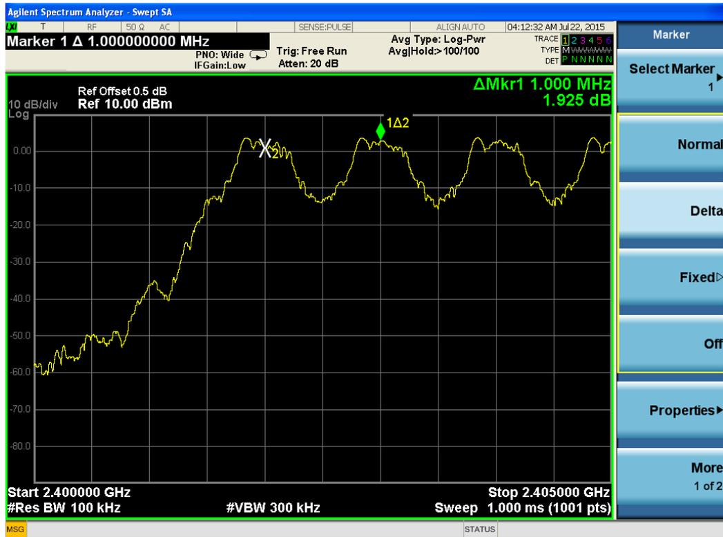
**Test Plot Of Frequency Separation (2Mbps)**
