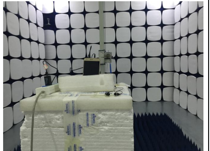
Radiated Spurious Emissions Test Setup Above 1GHz
