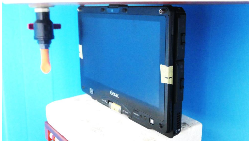
Setup for SAR Test (Body, Tablet mode, Top Side at 0 mm)
