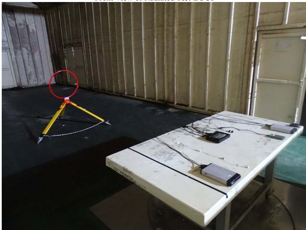
Front View of Radiated Test-LOOP
