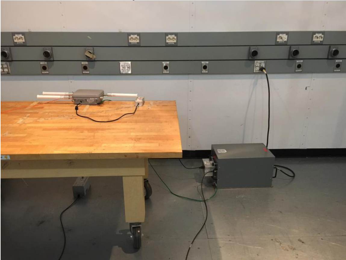
AC Mains Conducted Emissions setup
