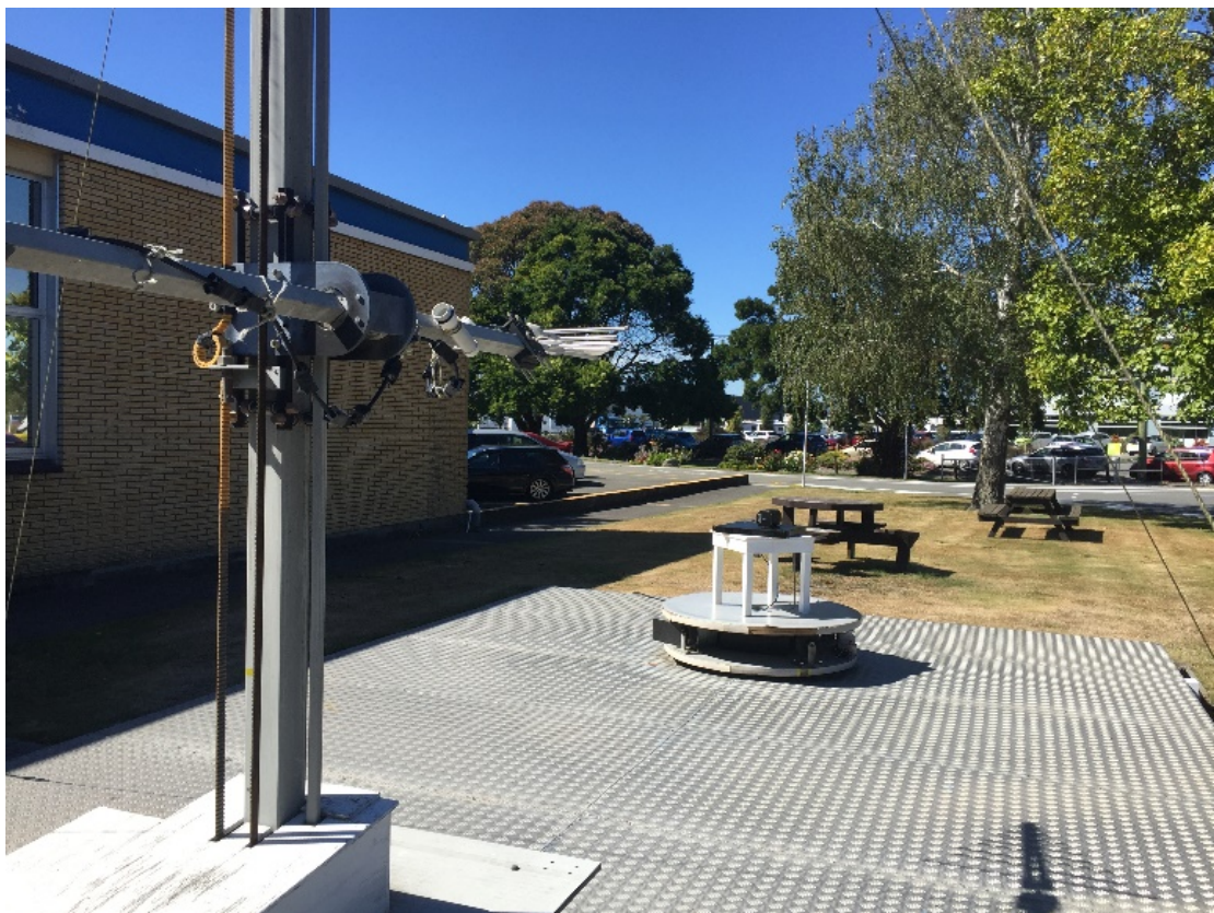
OATS RADIATED EMISSIONS SETUP
