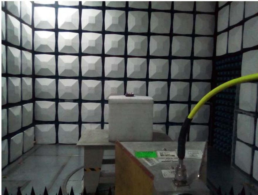
Radiated Emission View (Above 1GHz)
