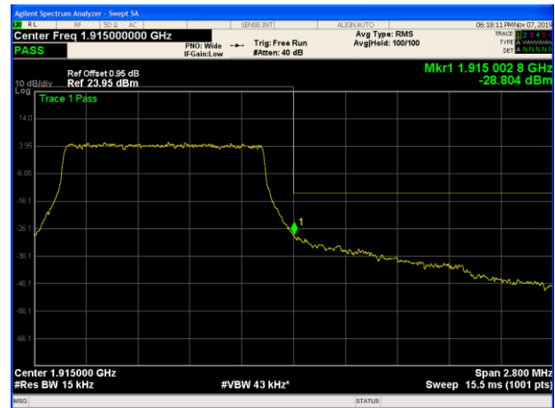
LTE Band 25 3MHz QPSK 1RB CH-High
