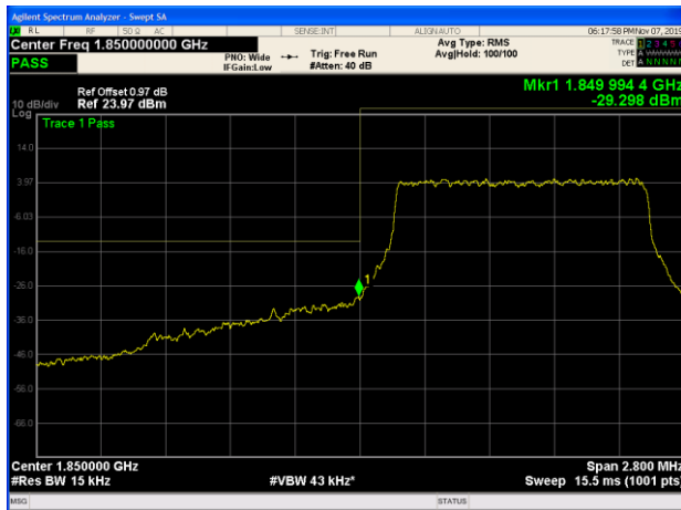
LTE Band 25 3MHz QPSK 1RB CH-Low
