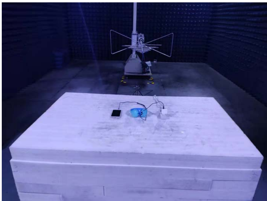
Photo of Radiated Emission Measurement Below 1GHz
