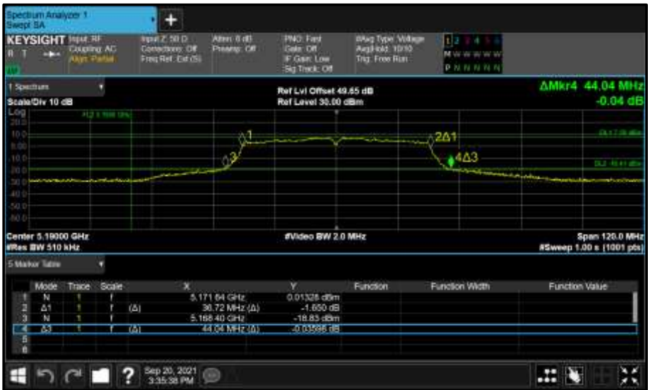
Figure 313 - Core 0 (A) 5190 MHz (CH38) 26 dB and 99% Bandwidth
