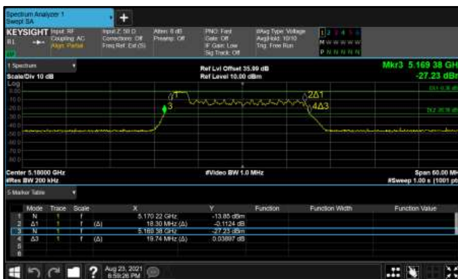
Figure 206 - Core 1 (B) 5180 MHz (CH36) 26 dB and 99% Bandwidth
