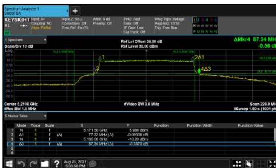
Figure 291 - Core 0 (A) 5210 MHz (CH42) 26 dB and 99% Bandwidth
