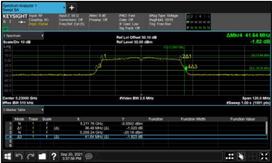
Figure 316 - Core 1 (B) 5230 MHz (CH46) 26 dB and 99% Bandwidth
