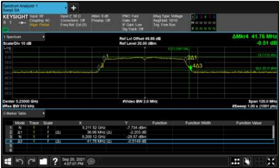
Figure 319 - Core 0 (A) 5230 MHz (CH46) 26 dB and 99% Bandwidth
