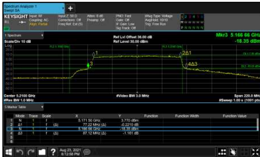
Figure 292 - Core 0 (A) 5210 MHz (CH42) 26 dB and 99% Bandwidth
