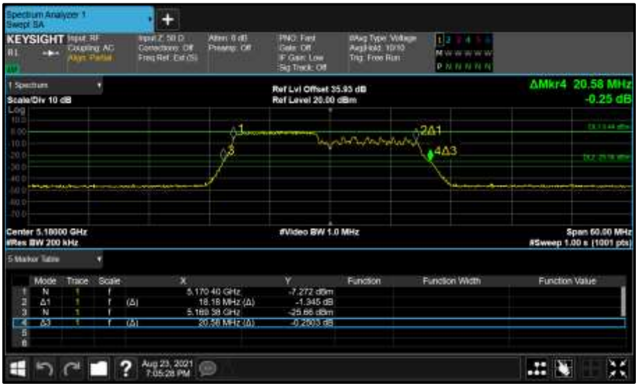
Figure 265 - Core 0 (A) 5180 MHz (CH36) 26 dB and 99% Bandwidth
