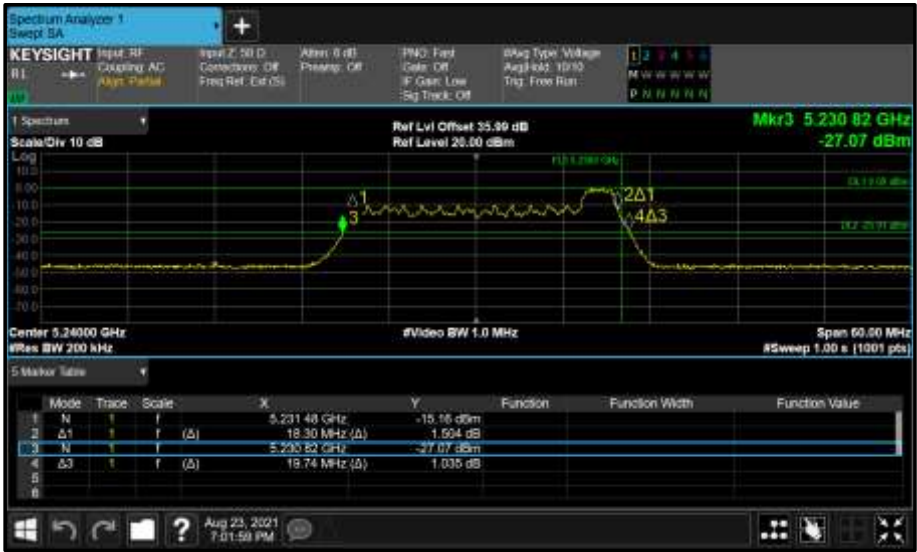
Figure 210 - Core 1 (B) 5240 MHz (CH48) 26 dB and 99% Bandwidth
