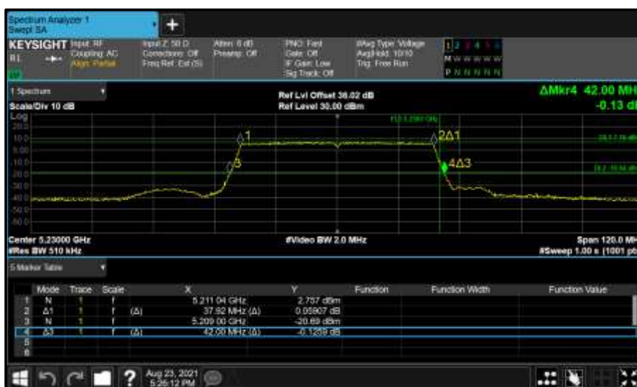
Figure 277 - Core 0 (A) 5230 MHz (CH46) 26 dB and 99% Bandwidth
