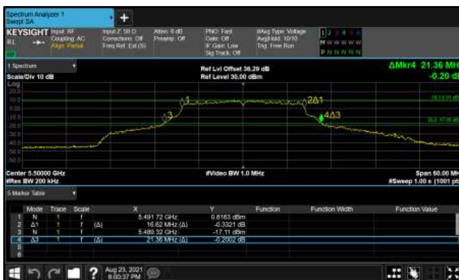
Figure 430 - Core 1 (B) 5500 MHz (CH100) 26 dB and 99% Bandwidth
