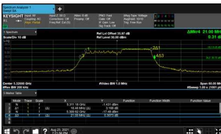
Figure 390 - Core 1 (B) 5320 MHz (CH64) 26 dB and 99% Bandwidth
