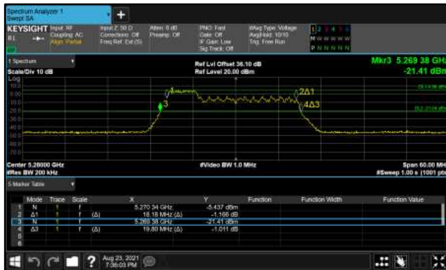
Figure 379 - Core 1 (B) 5280 MHz (CH56) 26 dB and 99% Bandwidth
