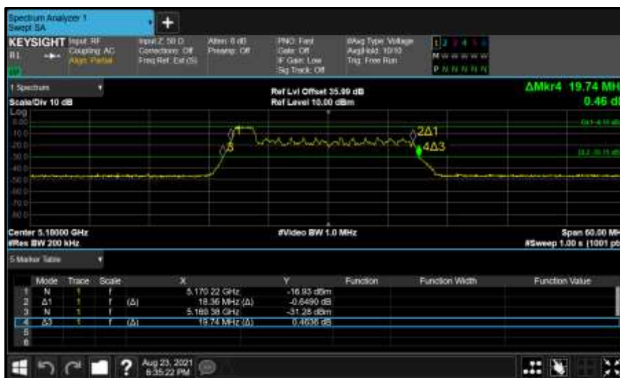
Figure 194 - Core 1 (B) 5180 MHz (CH36) 26 dB and 99% Bandwidth
