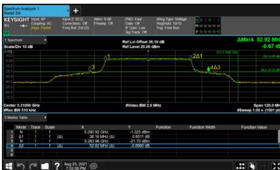
Figure 407 - Core 0 (A) 5310 MHz (CH62) 26 dB and 99% Bandwidth
