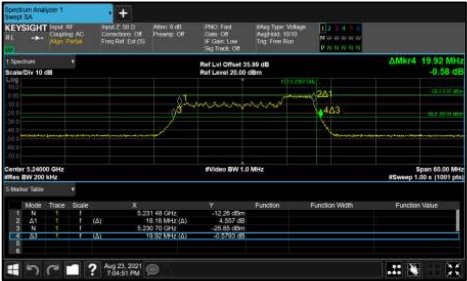
Figure 240 - Core 1 (B) 5240 MHz (CH48) 26 dB and 99% Bandwidth
