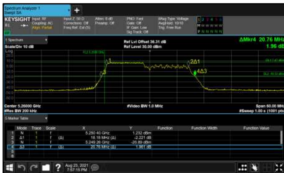
Figure 397 - Core 0 (A) 5260 MHz (CH52) 26 dB and 99% Bandwidth
