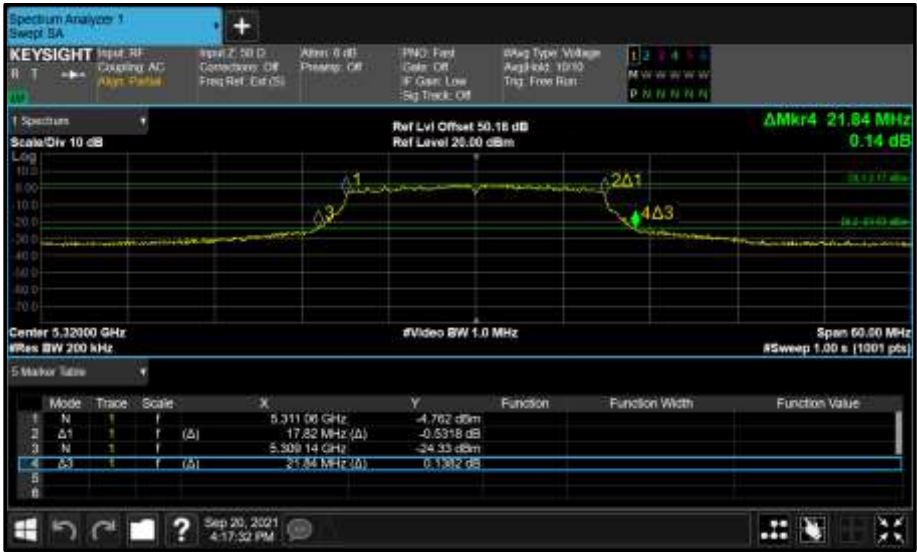
Figure 423 - Core 1 (B) 5320 MHz (CH64) 26 dB and 99% Bandwidth
