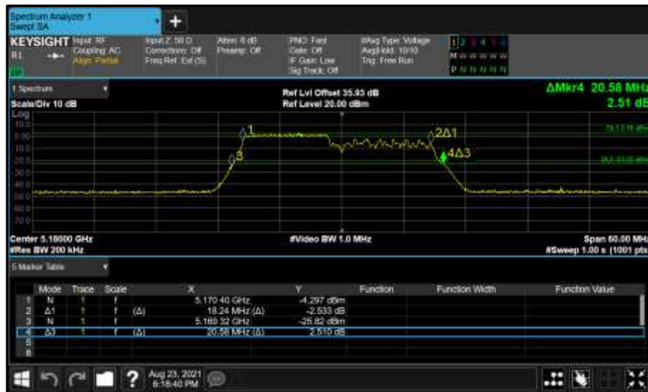
Figure 244 - Core 0 (A) 5180 MHz (CH36) 26 dB and 99% Bandwidth
