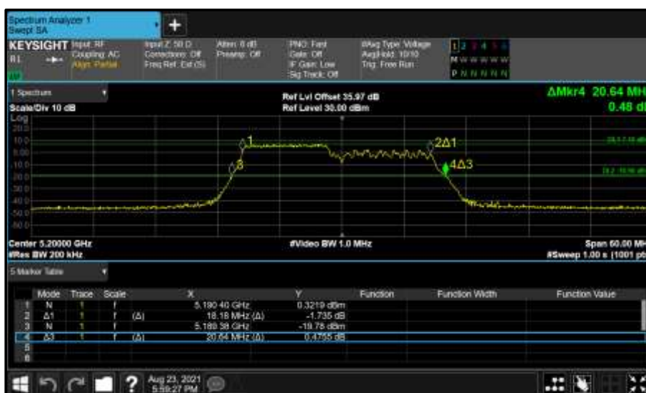
Figure 261 - Core 0 (A) 5200 MHz (CH40) 26 dB and 99% Bandwidth
