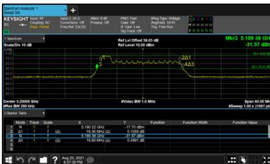
Figure 196 - Core 1 (B) 5200 MHz (CH40) 26 dB and 99% Bandwidth
