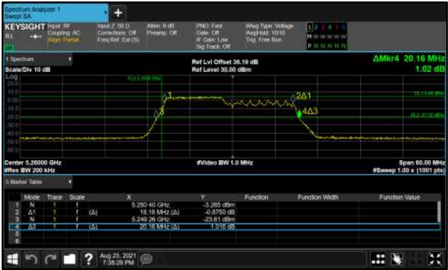
Figure 392 - Core 1 (B) 5260 MHz (CH52) 26 dB and 99% Bandwidth
