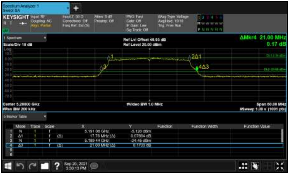
Figure 304 - Core 1 (B) 5200 MHz (CH40) 26 dB and 99% Bandwidth
