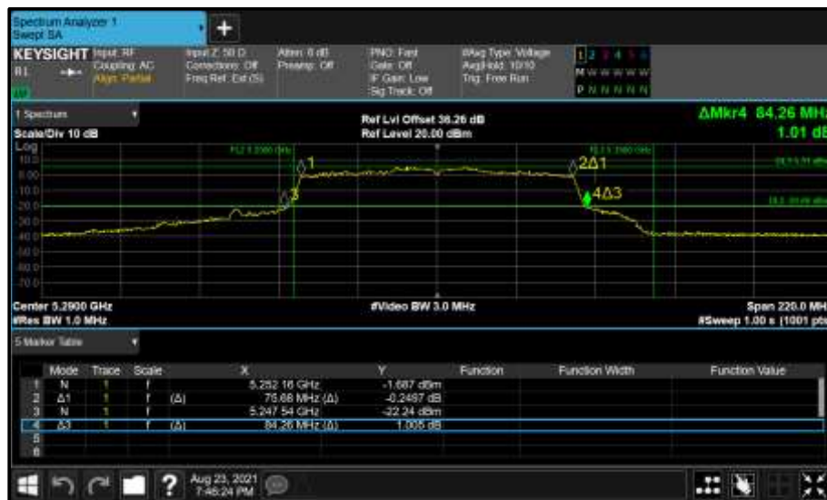
Figure 356 - Core 0 (A) 5290 MHz (CH58) 26 dB and 99% Bandwidth
