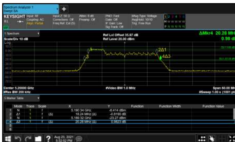
Figure 219 - Core 0 (A) 5200 MHz (CH40) 26 dB and 99% Bandwidth
