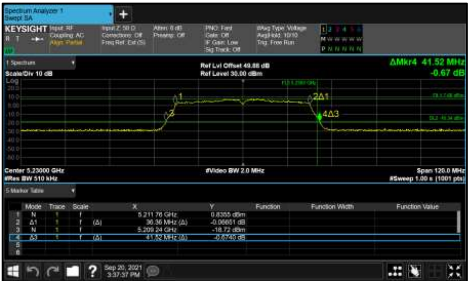
Figure 315 - Core 0 (A) 5230 MHz (CH46) 26 dB and 99% Bandwidth
