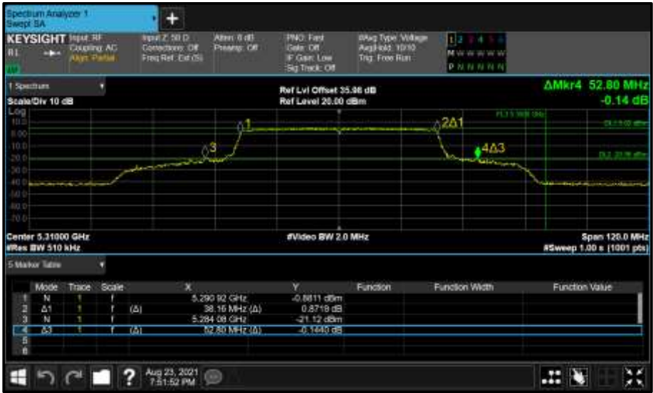
Figure 412 - Core 1 (B) 5310 MHz (CH62) 26 dB and 99% Bandwidth
