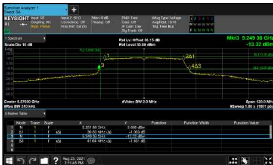
Figure 343 - Core 1 (B) 5270 MHz (CH54) 26 dB and 99% Bandwidth
