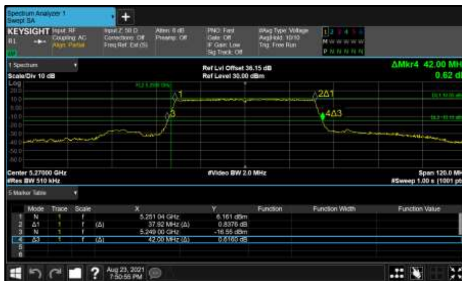
Figure 410 - Core 1 (B) 5270 MHz (CH54) 26 dB and 99% Bandwidth
