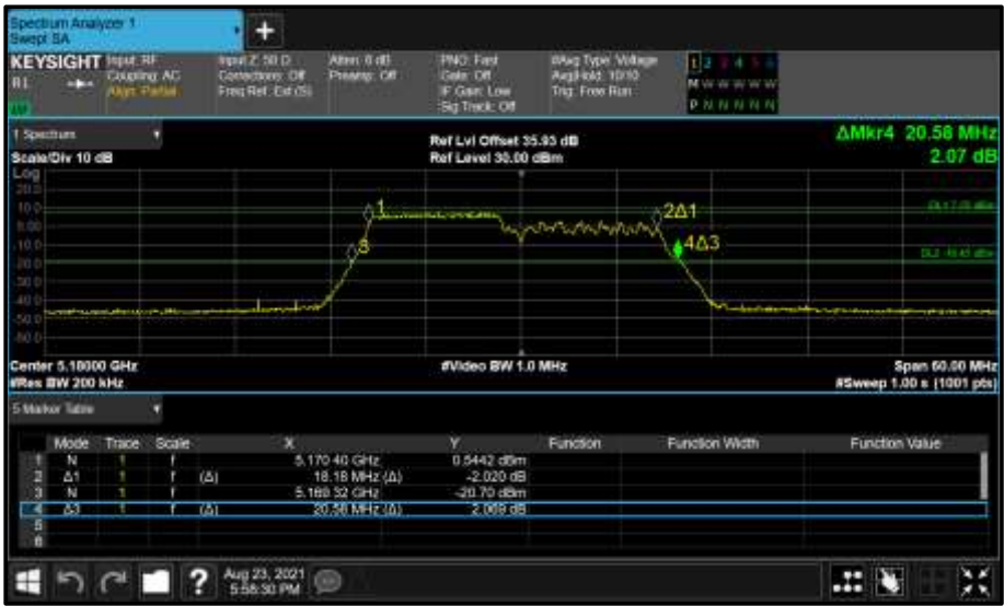
Figure 259 - Core 0 (A) 5180 MHz (CH36) 26 dB and 99% Bandwidth
