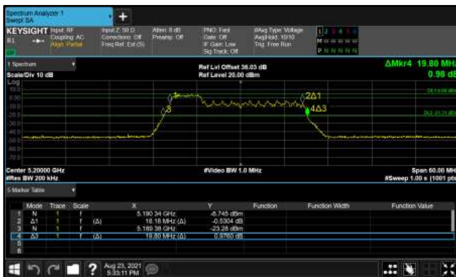
Figure 220 - Core 1 (B) 5200 MHz (CH40) 26 dB and 99% Bandwidth
