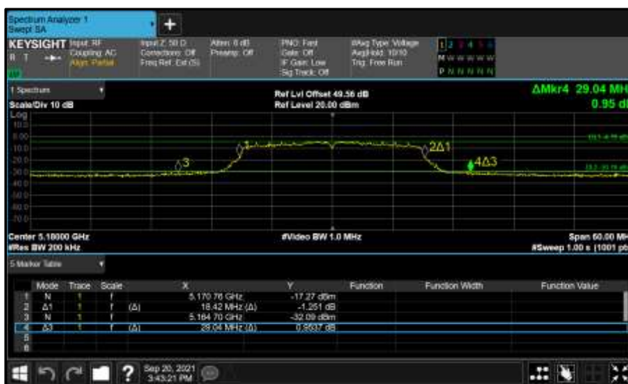
Figure 307 - Core 0 (A) 5180 MHz (CH36) 26 dB and 99% Bandwidth
