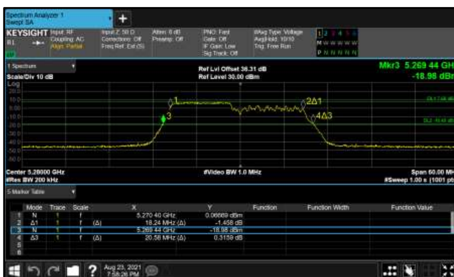
Figure 399 - Core 0 (A) 5280 MHz (CH56) 26 dB and 99% Bandwidth
