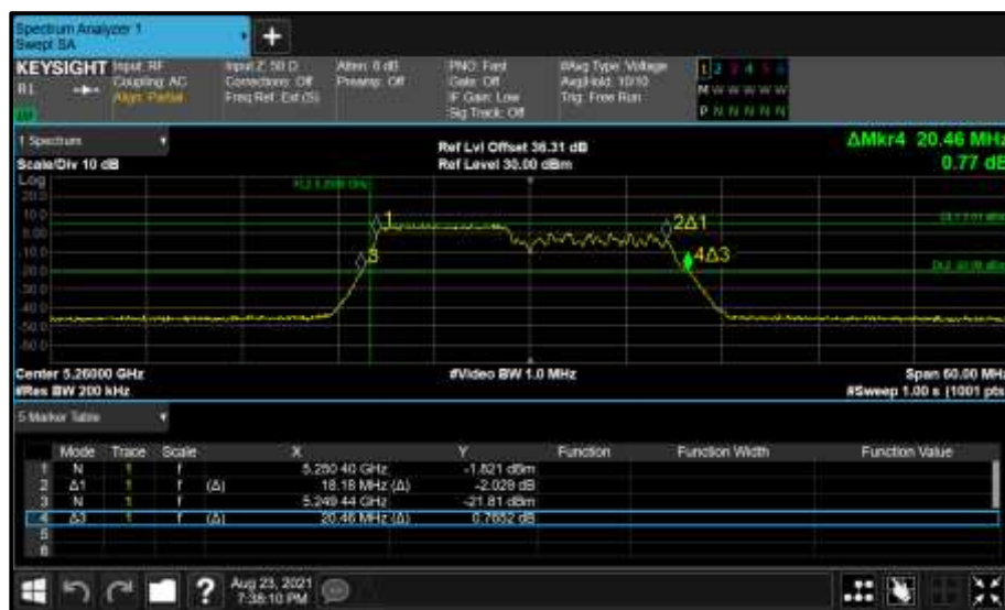
Figure 391 - Core 0 (A) 5260 MHz (CH52) 26 dB and 99% Bandwidth
