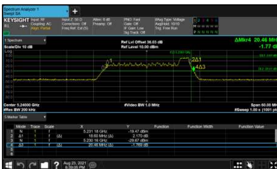
Figure 197 - Core 0 (A) 5240 MHz (CH48) 26 dB and 99% Bandwidth
