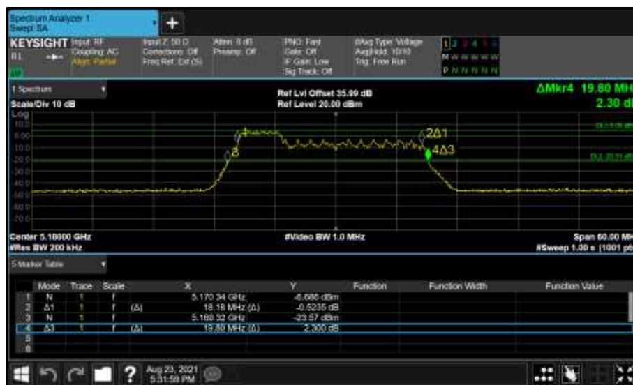
Figure 218 - Core 1 (B) 5180 MHz (CH36) 26 dB and 99% Bandwidth
