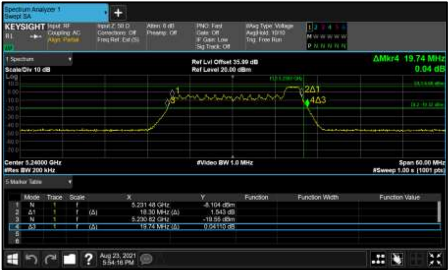
Figure 204 - Core 1 (B) 5240 MHz (CH48) 26 dB and 99% Bandwidth
