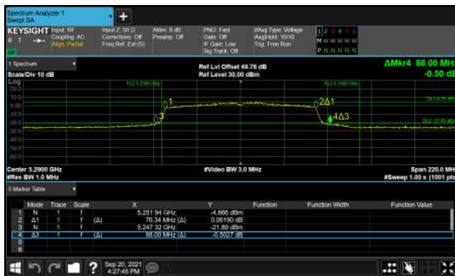
Figure 428 - Core 0 (A) 5290 MHz (CH58) 26 dB and 99% Bandwidth
