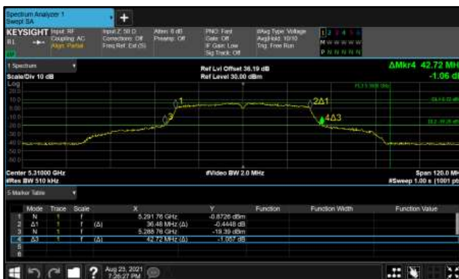
Figure 347 - Core 0 (A) 5310 MHz (CH62) 26 dB and 99% Bandwidth
