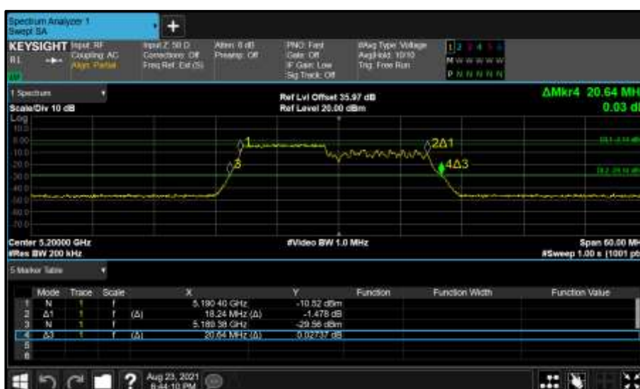
Figure 255 - Core 0 (A) 5200 MHz (CH40) 26 dB and 99% Bandwidth
