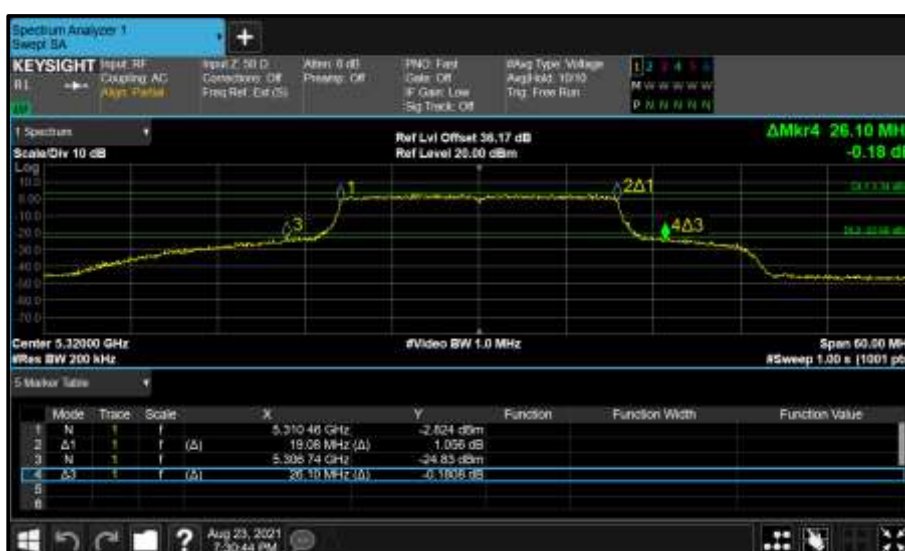
Figure 365 - Core 0 (A) 5320 MHz (CH64) 26 dB and 99% Bandwidth
