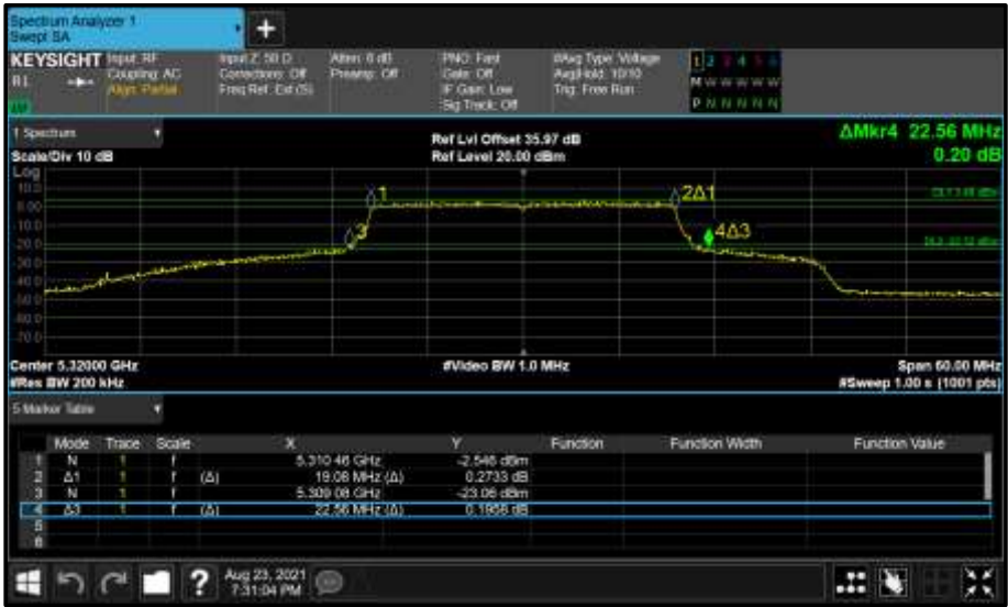
Figure 366 - Core 1 (B) 5320 MHz (CH64) 26 dB and 99% Bandwidth
