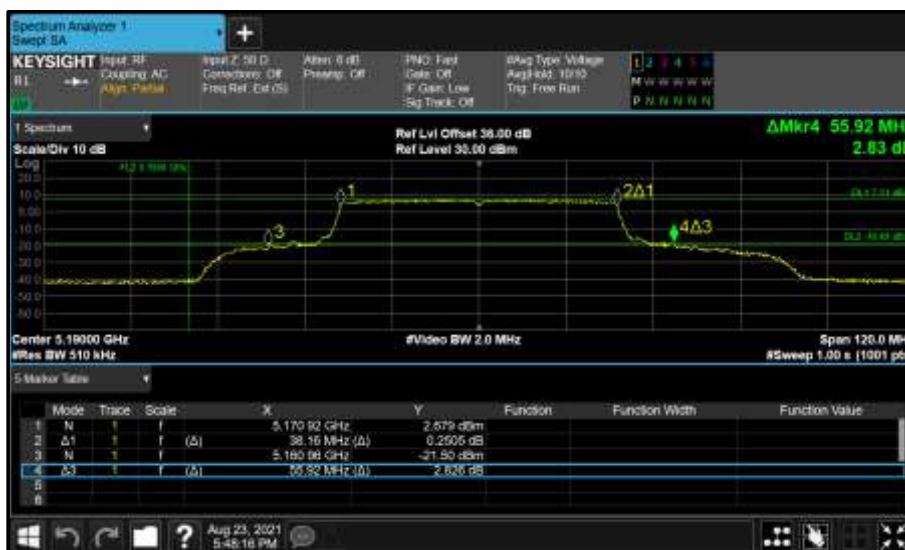
Figure 284 - Core 1 (B) 5190 MHz (CH38) 26 dB and 99% Bandwidth
