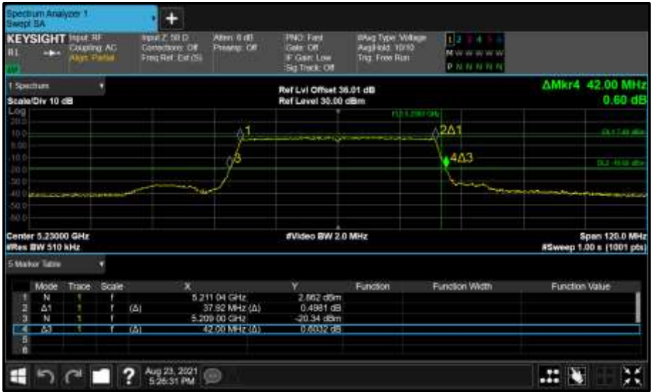
Figure 278 - Core 1 (B) 5230 MHz (CH46) 26 dB and 99% Bandwidth
