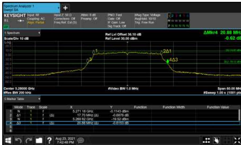
Figure 340 - Core 1 (B) 5280 MHz (CH56) 26 dB and 99% Bandwidth
