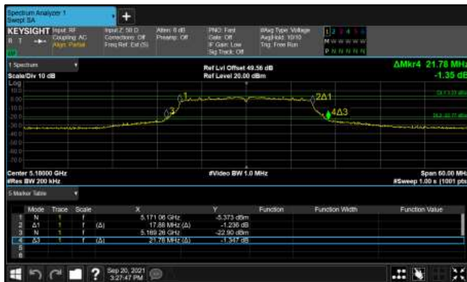
Figure 301 - Core 0 (A) 5180 MHz (CH36) 26 dB and 99% Bandwidth
