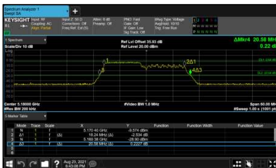
Figure 253 - Core 0 (A) 5180 MHz (CH36) 26 dB and 99% Bandwidth
