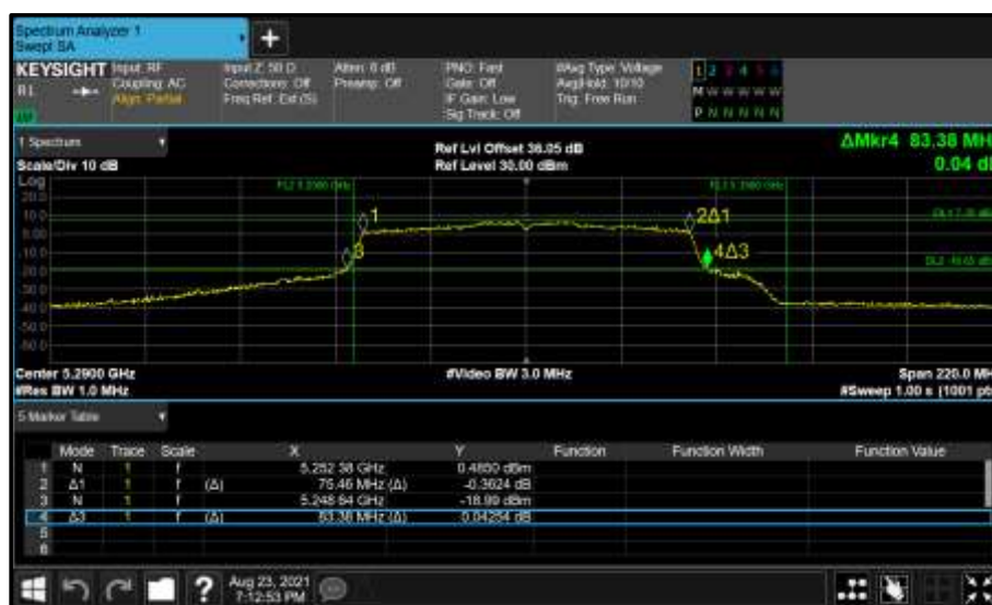
Figure 353 - Core 1 (B) 5290 MHz (CH58) 26 dB and 99% Bandwidth
