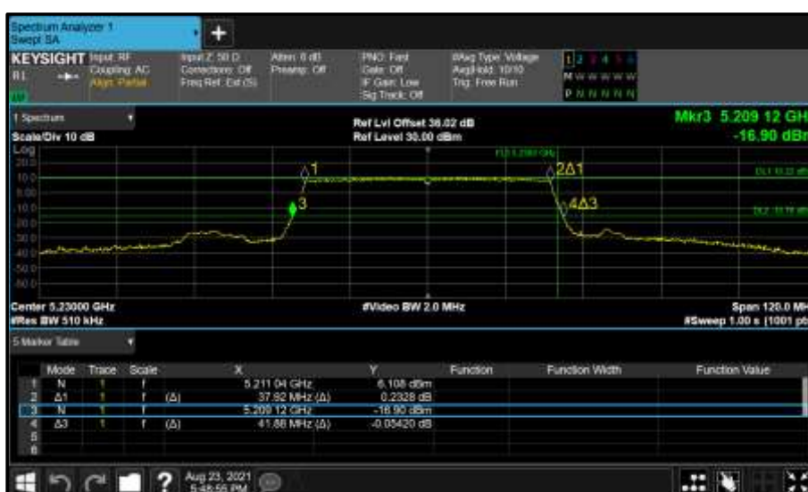
Figure 285 - Core 0 (A) 5230 MHz (CH46) 26 dB and 99% Bandwidth
