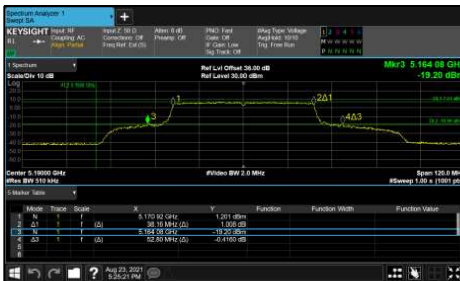
Figure 276 - Core 1 (B) 5190 MHz (CH38) 26 dB and 99% Bandwidth
