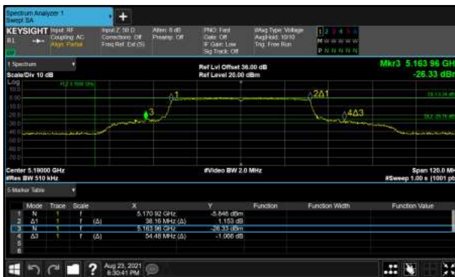
Figure 280 - Core 1 (B) 5190 MHz (CH38) 26 dB and 99% Bandwidth
