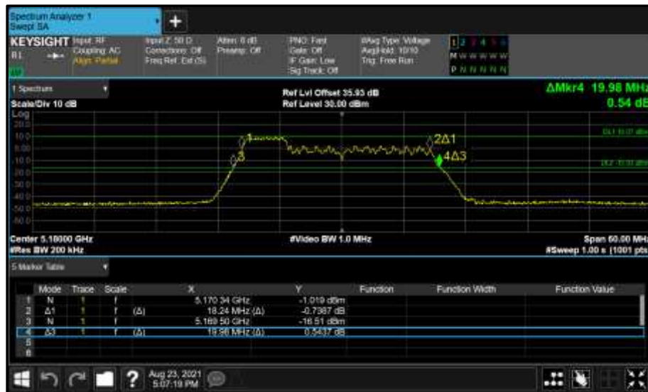
Figure 211 - Core 0 (A) 5180 MHz (CH36) 26 dB and 99% Bandwidth
