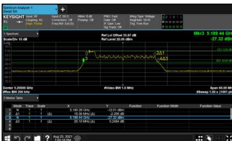
Figure 207 - Core 0 (A) 5200 MHz (CH40) 26 dB and 99% Bandwidth
