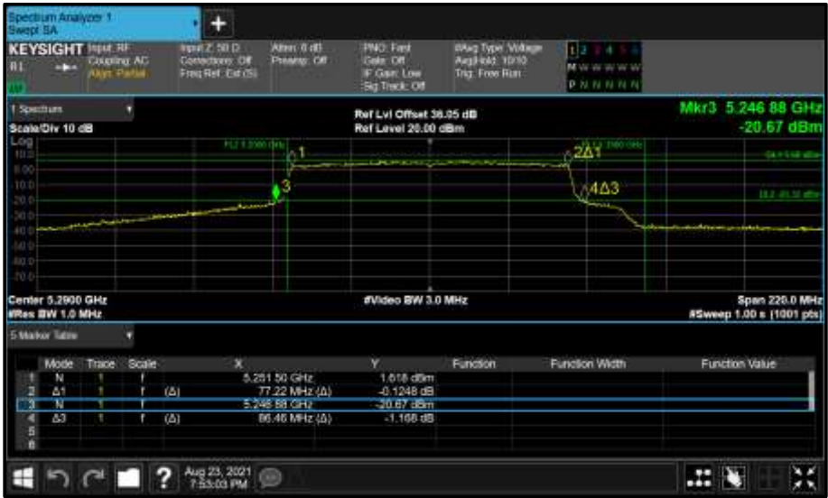
Figure 417 - Core 1 (B) 5290 MHz (CH58) 26 dB and 99% Bandwidth
