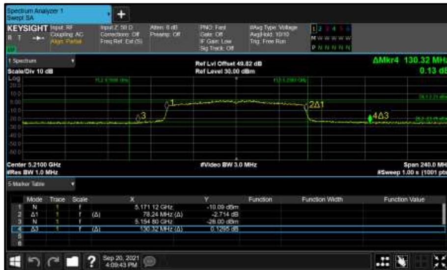
Figure 323 - Core 0 (A) 5210 MHz (CH42) 26 dB and 99% Bandwidth
