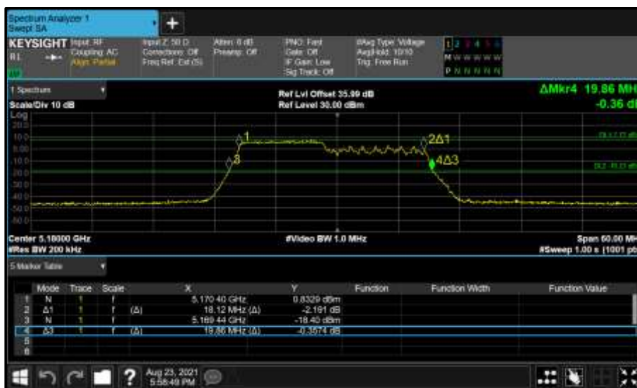
Figure 260 - Core 1 (B) 5180 MHz (CH36) 26 dB and 99% Bandwidth
