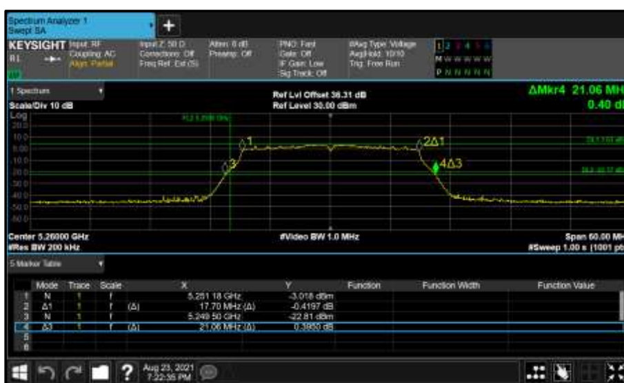
Figure 331 - Core 0 (A) 5260 MHz (CH52) 26 dB and 99% Bandwidth
