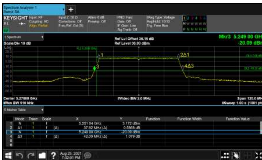
Figure 406 - Core 1 (B) 5270 MHz (CH54) 26 dB and 99% Bandwidth
