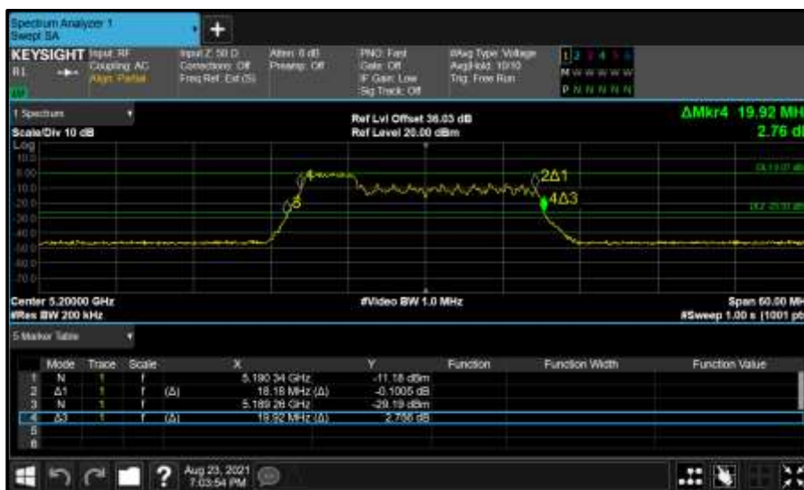
Figure 238 - Core 1 (B) 5200 MHz (CH40) 26 dB and 99% Bandwidth
