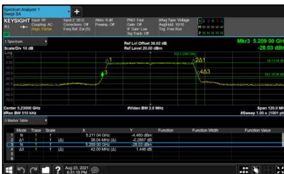
Figure 281 - Core 0 (A) 5230 MHz (CH46) 26 dB and 99% Bandwidth
