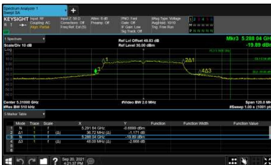
Figure 426 - Core 0 (A) 5310 MHz (CH62) 26 dB and 99% Bandwidth
