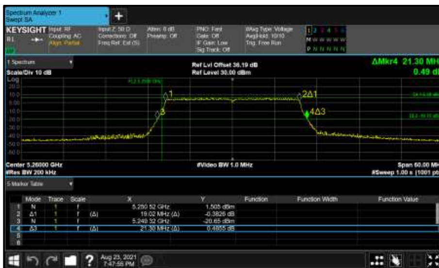
Figure 368 - Core 1 (B) 5260 MHz (CH52) 26 dB and 99% Bandwidth
