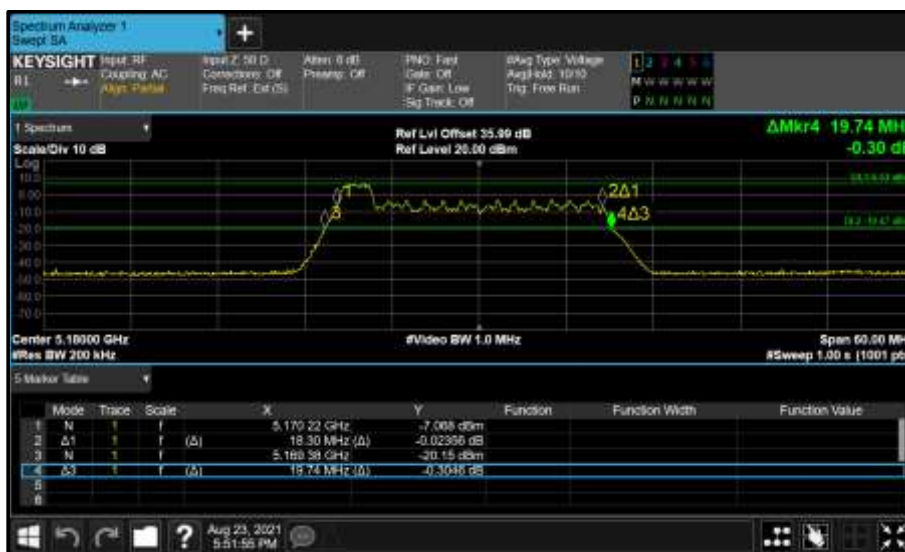
Figure 200 - Core 1 (B) 5180 MHz (CH36) 26 dB and 99% Bandwidth
