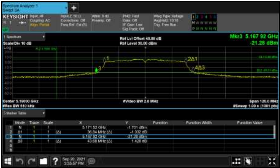
Figure 314 - Core 1 (B) 5190 MHz (CH38) 26 dB and 99% Bandwidth
