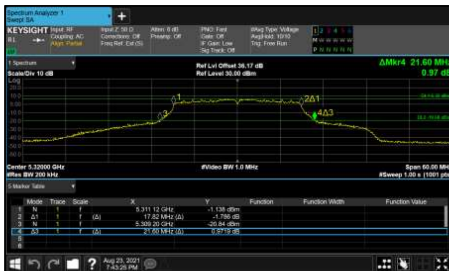
Figure 341 - Core 0 (A) 5320 MHz (CH64) 26 dB and 99% Bandwidth
