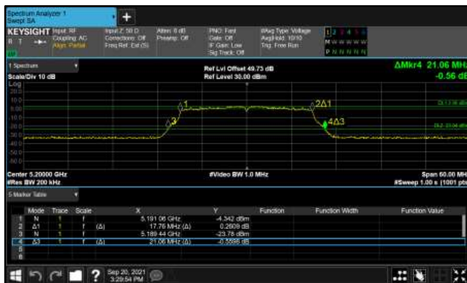
Figure 303 - Core 0 (A) 5200 MHz (CH40) 26 dB and 99% Bandwidth
