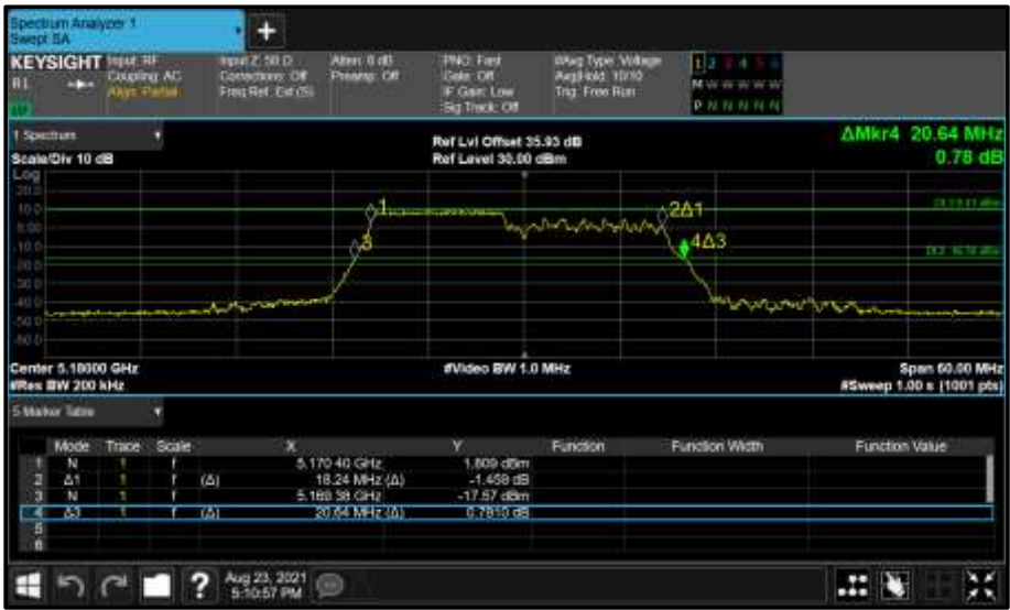
Figure 241 - Core 0 (A) 5180 MHz (CH36) 26 dB and 99% Bandwidth
