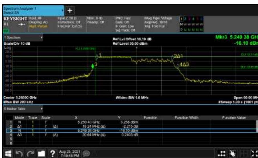
Figure 388 - Core 1 (B) 5260 MHz (CH52) 26 dB and 99% Bandwidth
