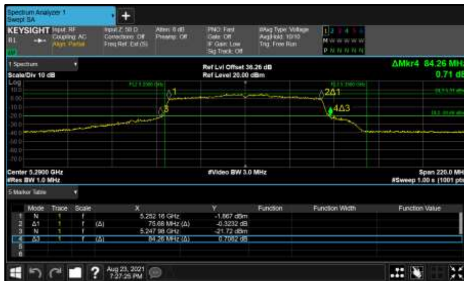
Figure 354 - Core 0 (A) 5290 MHz (CH58) 26 dB and 99% Bandwidth
