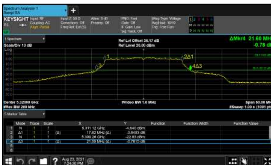
Figure 335 - Core 0 (A) 5320 MHz (CH64) 26 dB and 99% Bandwidth
