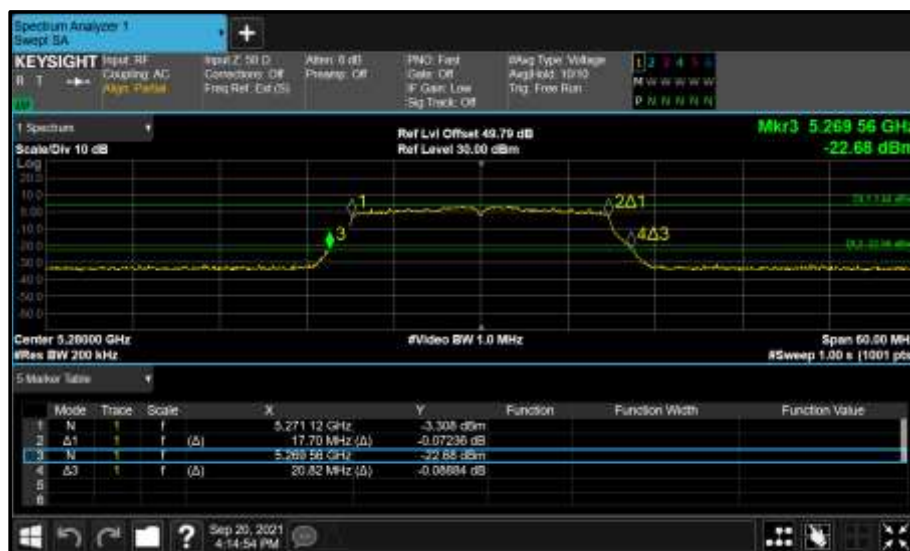
Figure 420 - Core 0 (A) 5280 MHz (CH56) 26 dB and 99% Bandwidth
