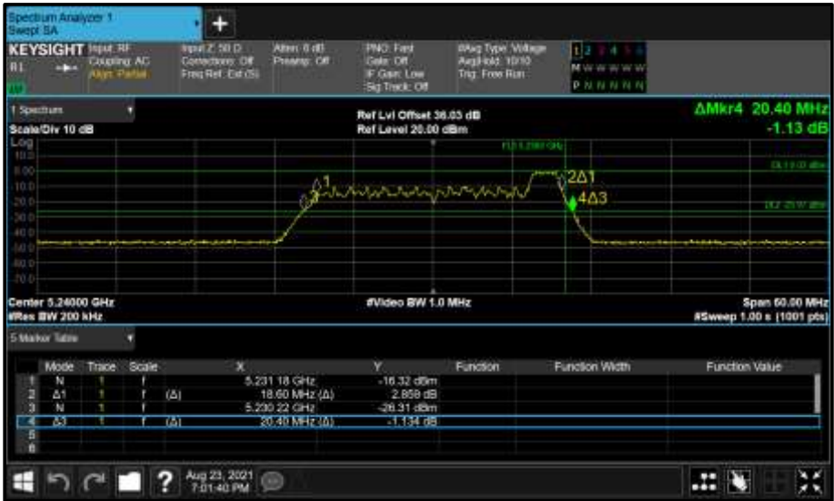
Figure 209 - Core 0 (A) 5240 MHz (CH48) 26 dB and 99% Bandwidth
