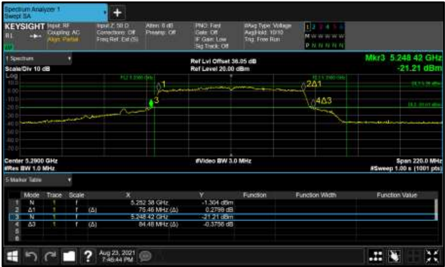
Figure 357 - Core 1 (B) 5290 MHz (CH58) 26 dB and 99% Bandwidth
