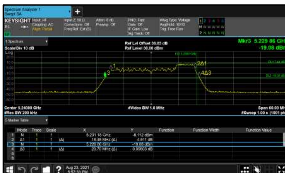
Figure 233 - Core 0 (A) 5240 MHz (CH48) 26 dB and 99% Bandwidth
