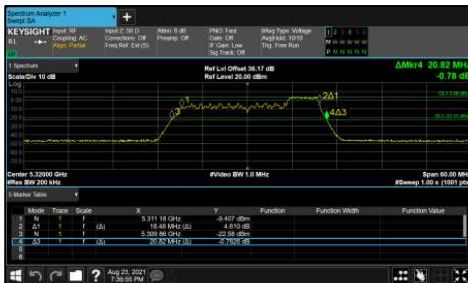
Figure 380 - Core 0 (A) 5320 MHz (CH64) 26 dB and 99% Bandwidth
