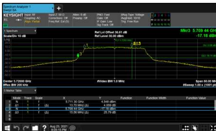
Figure 437 - Core 1 (B) 5720 MHz (CH144) 26 dB and 99% Bandwidth
