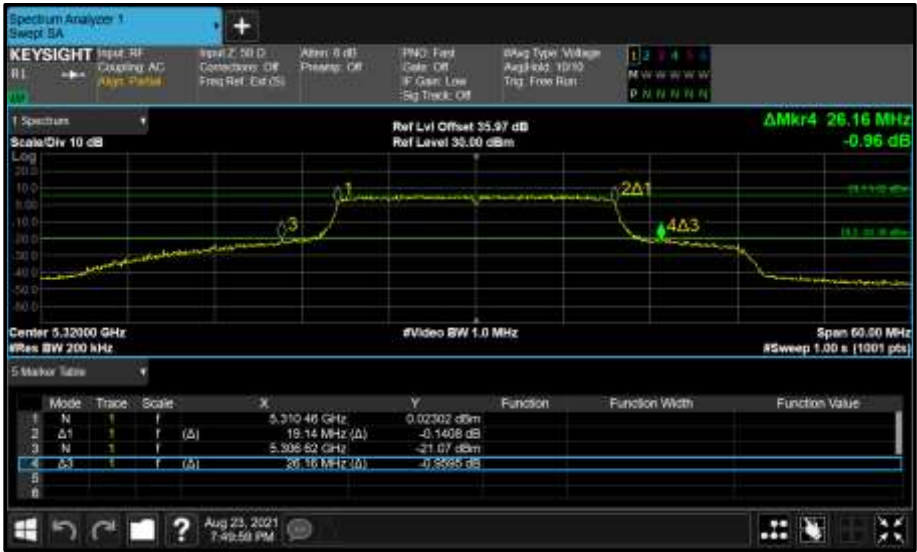
Figure 372 - Core 1 (B) 5320 MHz (CH64) 26 dB and 99% Bandwidth
