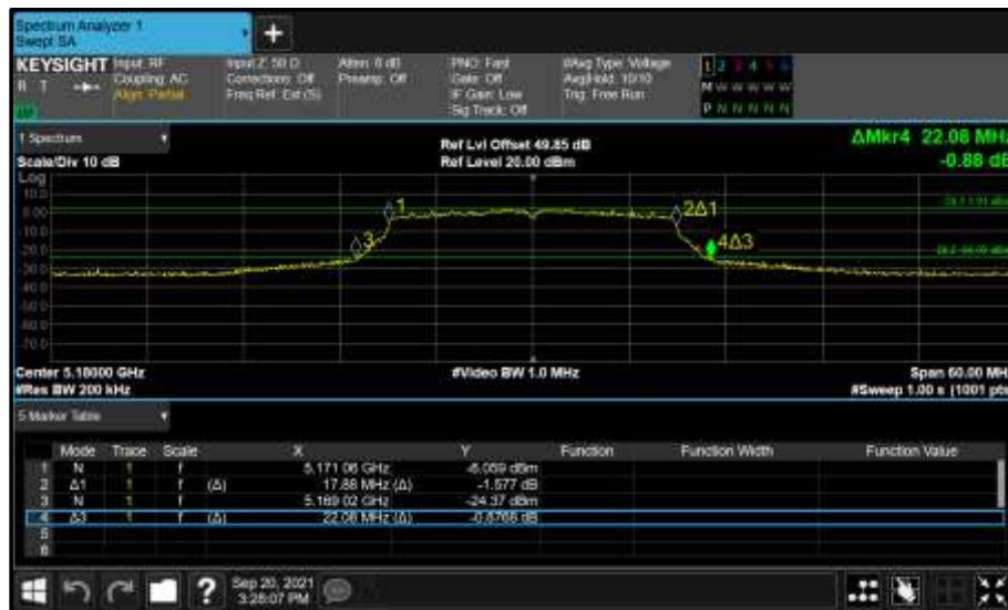
Figure 302 - Core 1 (B) 5180 MHz (CH36) 26 dB and 99% Bandwidth
