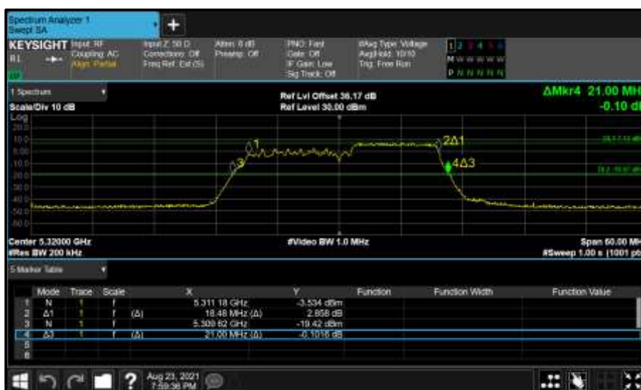
Figure 401 - Core 0 (A) 5320 MHz (CH64) 26 dB and 99% Bandwidth
