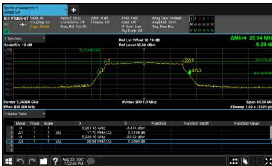
Figure 332 - Core 1 (B) 5260 MHz (CH52) 26 dB and 99% Bandwidth
