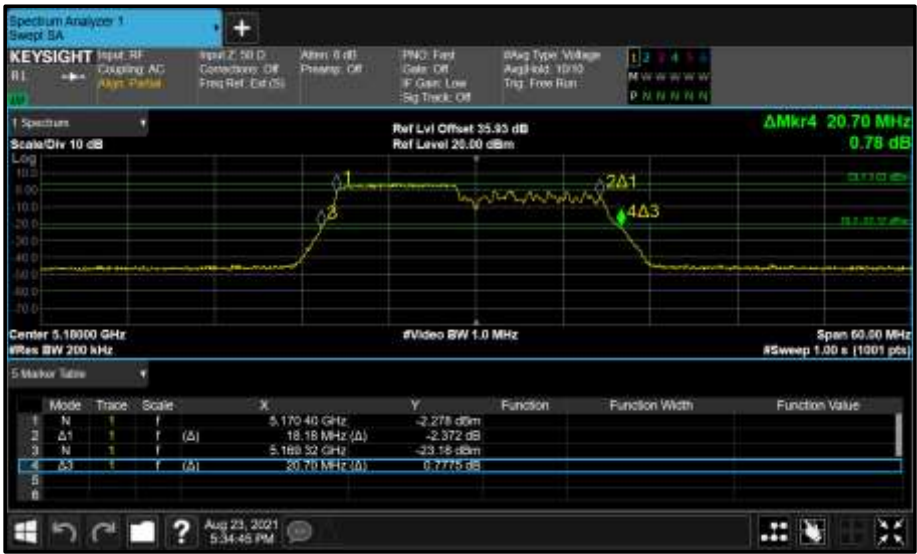
Figure 247 - Core 0 (A) 5180 MHz (CH36) 26 dB and 99% Bandwidth
