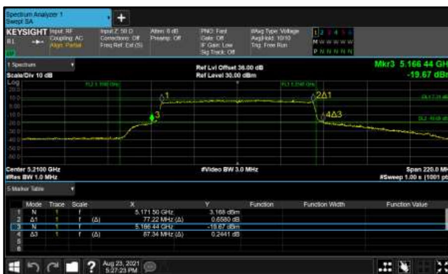
Figure 293 - Core 0 (A) 5210 MHz (CH42) 26 dB and 99% Bandwidth
