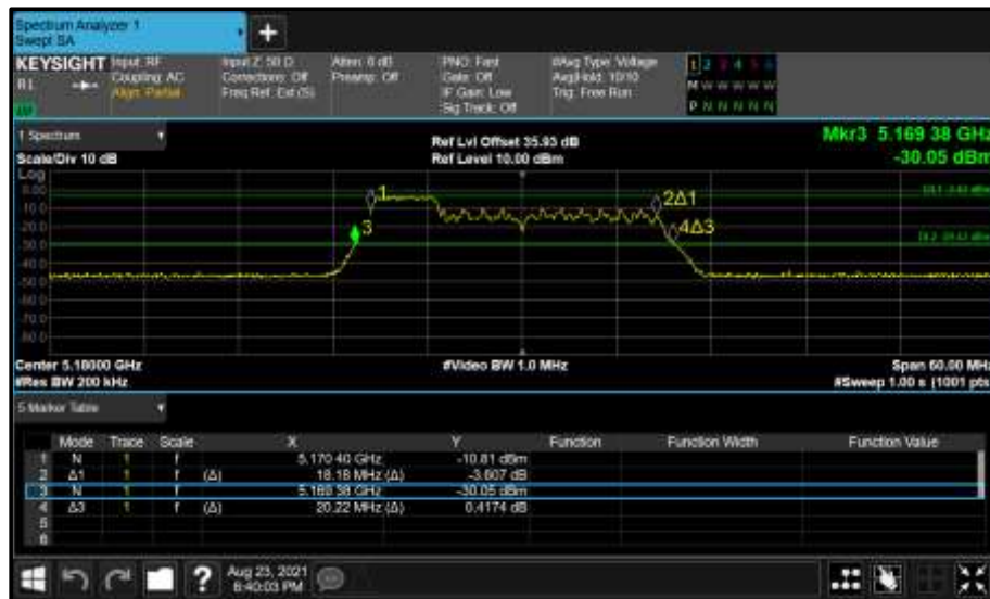
Figure 223 - Core 0 (A) 5180 MHz (CH36) 26 dB and 99% Bandwidth
