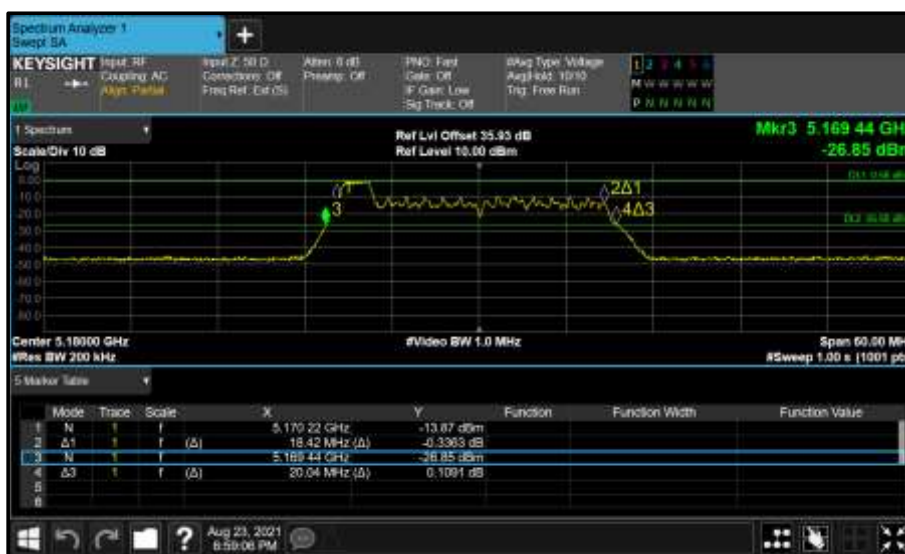
Figure 205 - Core 0 (A) 5180 MHz (CH36) 26 dB and 99% Bandwidth
