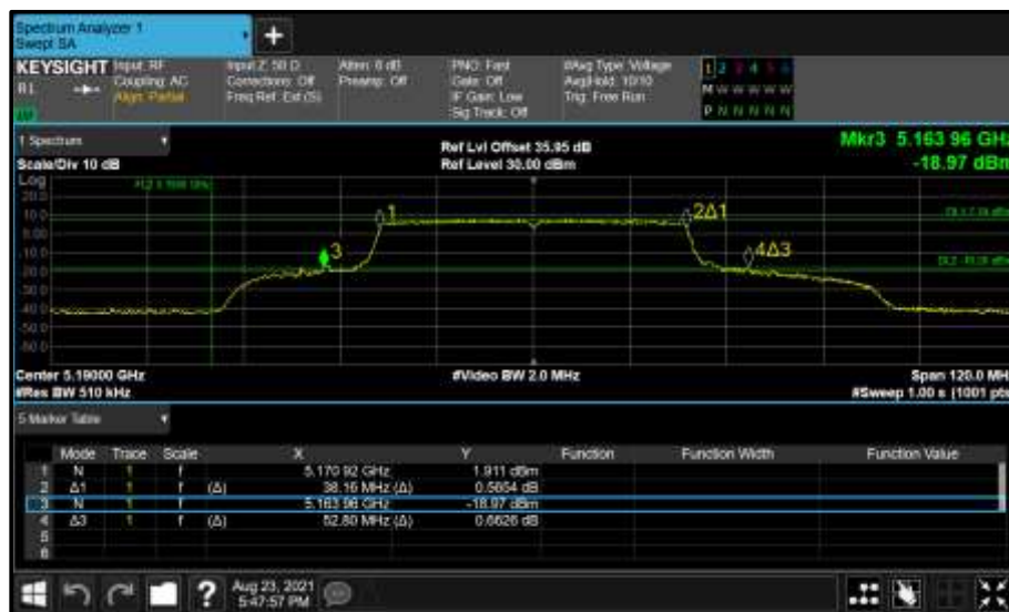
Figure 283 - Core 0 (A) 5190 MHz (CH38) 26 dB and 99% Bandwidth
