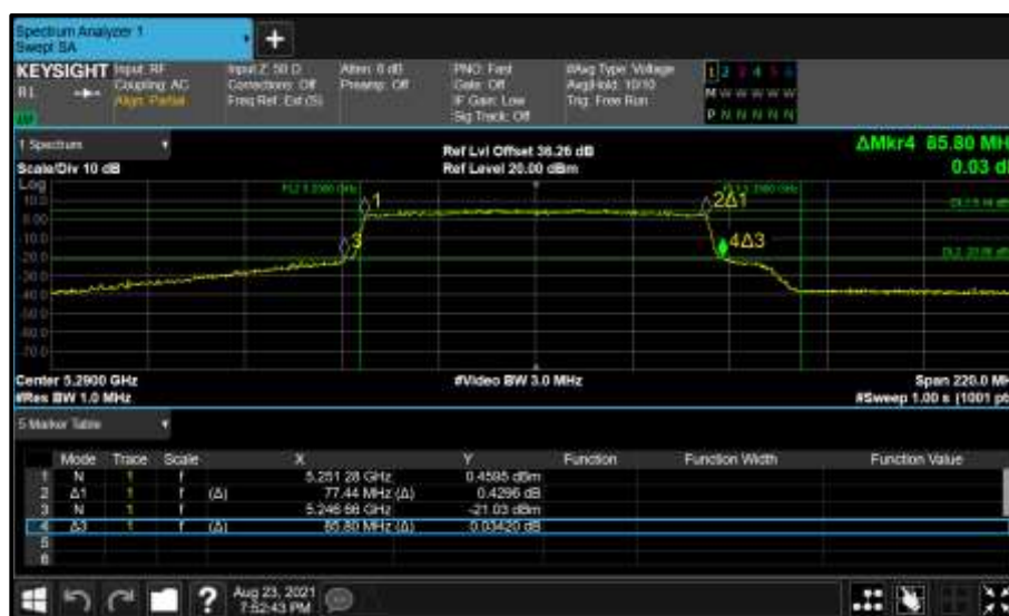
Figure 416 - Core 0 (A) 5290 MHz (CH58) 26 dB and 99% Bandwidth
