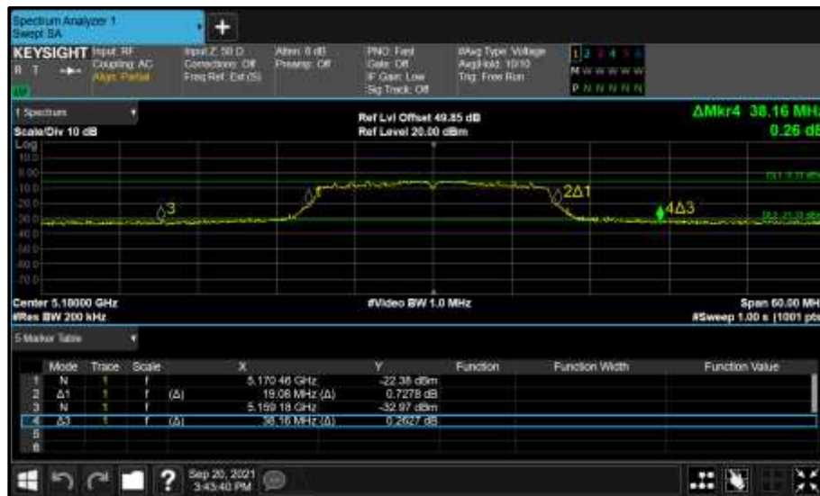
Figure 308 - Core 1 (B) 5180 MHz (CH36) 26 dB and 99% Bandwidth
