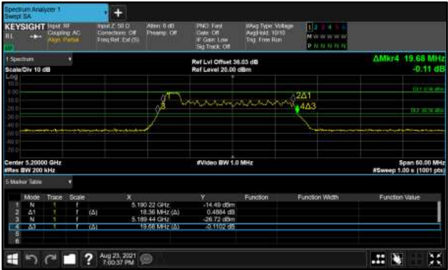
Figure 208 - Core 1 (B) 5200 MHz (CH40) 26 dB and 99% Bandwidth
