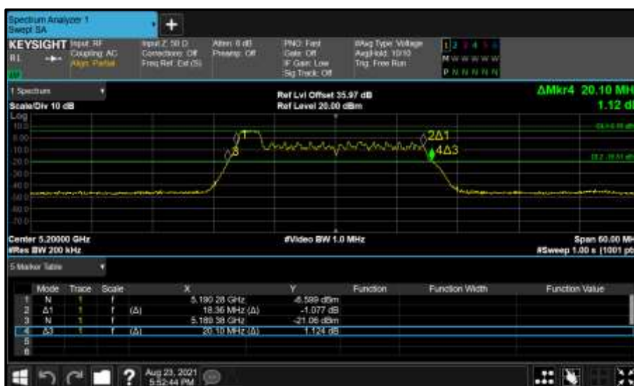
Figure 201 - Core 0 (A) 5200 MHz (CH40) 26 dB and 99% Bandwidth
