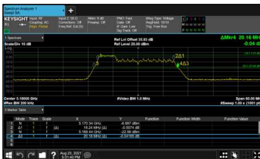
Figure 217 - Core 0 (A) 5180 MHz (CH36) 26 dB and 99% Bandwidth
