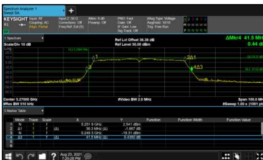
Figure 345 - Core 0 (A) 5270 MHz (CH54) 26 dB and 99% Bandwidth
