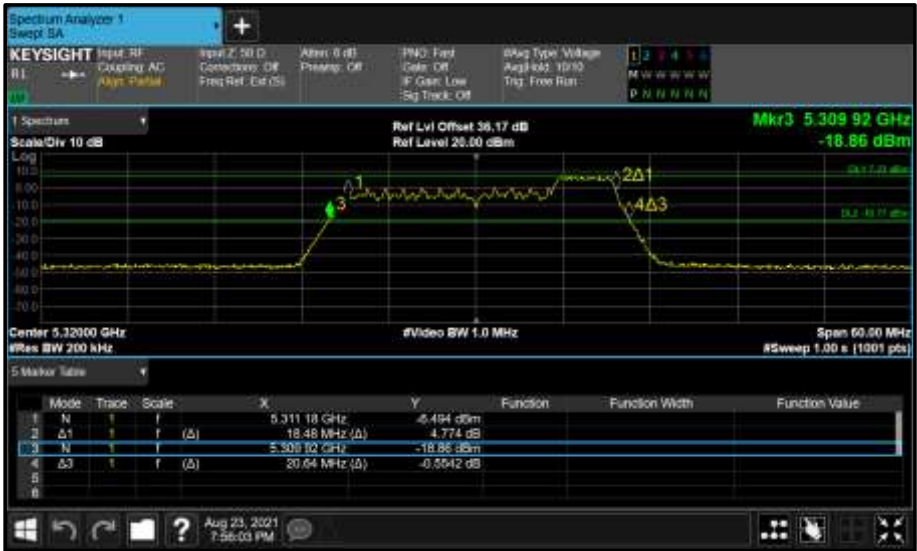
Figure 386 - Core 0 (A) 5320 MHz (CH64) 26 dB and 99% Bandwidth
