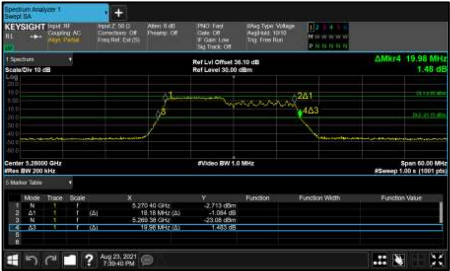
Figure 394 - Core 1 (B) 5280 MHz (CH56) 26 dB and 99% Bandwidth
