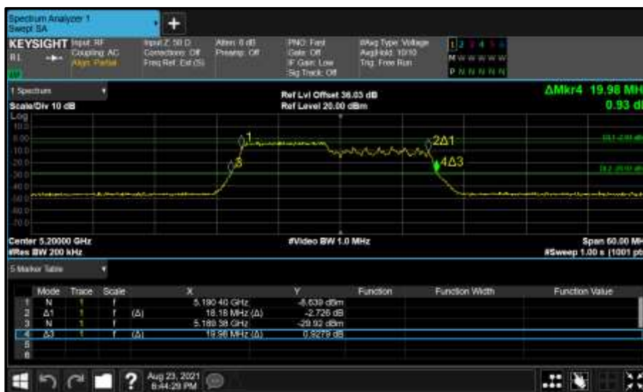
Figure 256 - Core 1 (B) 5200 MHz (CH40) 26 dB and 99% Bandwidth
