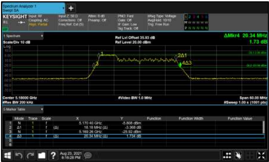
Figure 214 - Core 0 (A) 5180 MHz (CH36) 26 dB and 99% Bandwidth
