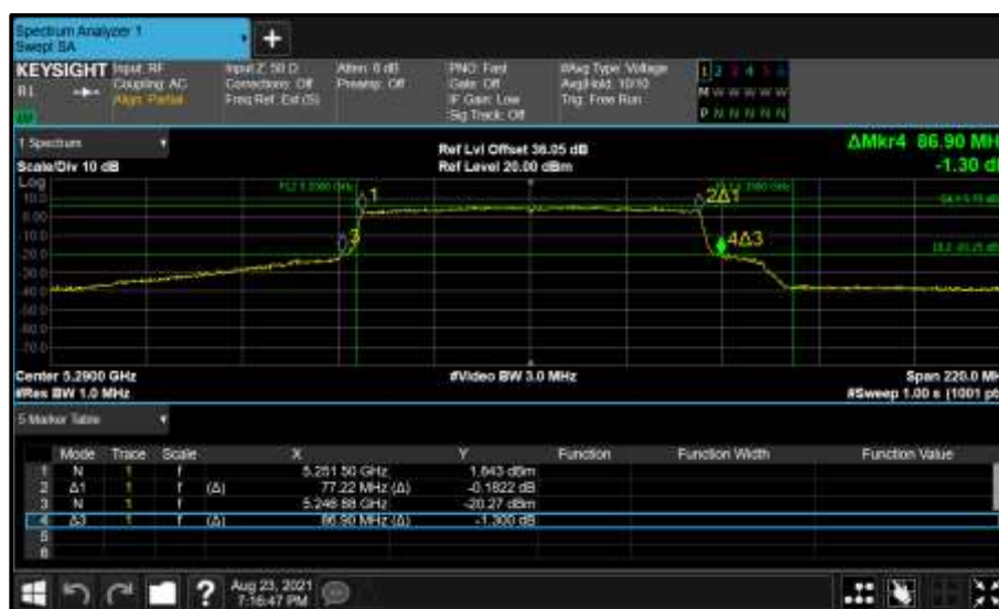
Figure 413 - Core 1 (B) 5290 MHz (CH58) 26 dB and 99% Bandwidth
