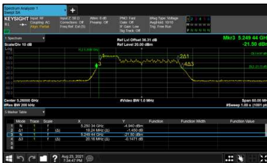
Figure 376 - Core 0 (A) 5260 MHz (CH52) 26 dB and 99% Bandwidth
