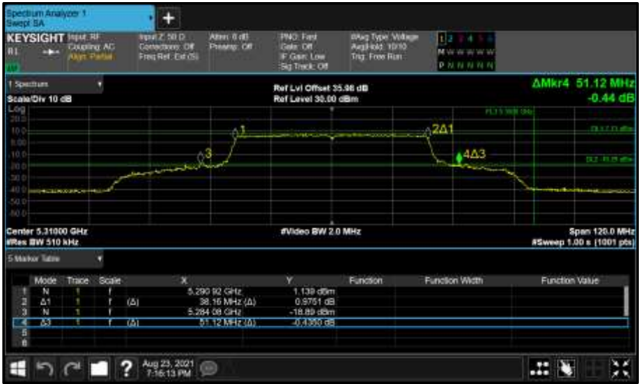
Figure 404 - Core 1 (B) 5310 MHz (CH62) 26 dB and 99% Bandwidth
