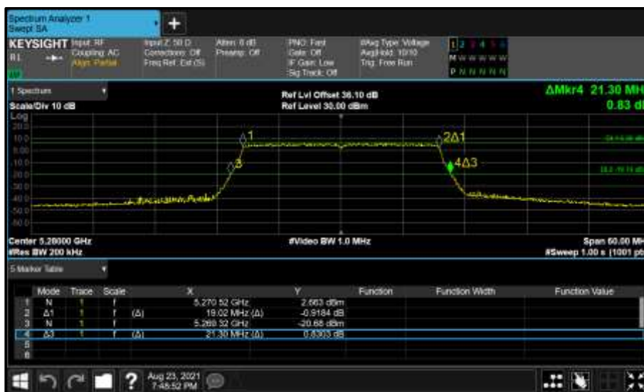
Figure 370 - Core 1 (B) 5280 MHz (CH56) 26 dB and 99% Bandwidth
