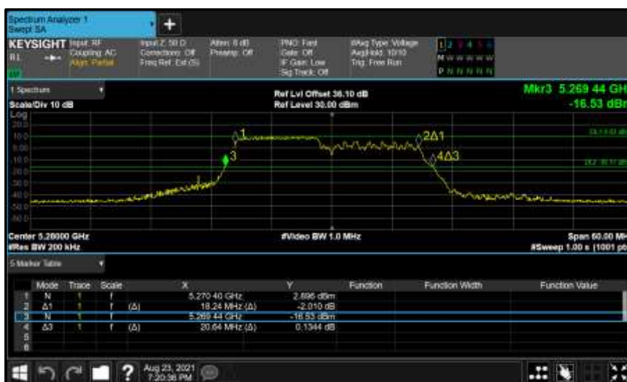
Figure 389 - Core 1 (B) 5280 MHz (CH56) 26 dB and 99% Bandwidth
