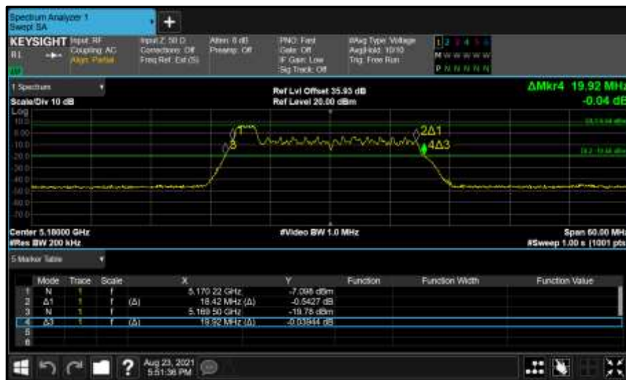
Figure 199 - Core 0 (A) 5180 MHz (CH36) 26 dB and 99% Bandwidth
