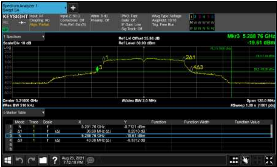
Figure 344 - Core 1 (B) 5310 MHz (CH62) 26 dB and 99% Bandwidth
