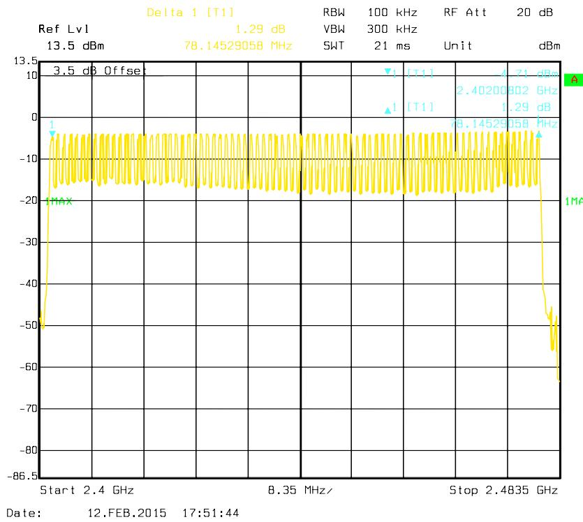
**EDR ( $\pi/4$ -DQPSK): Number of Hopping Channels**
