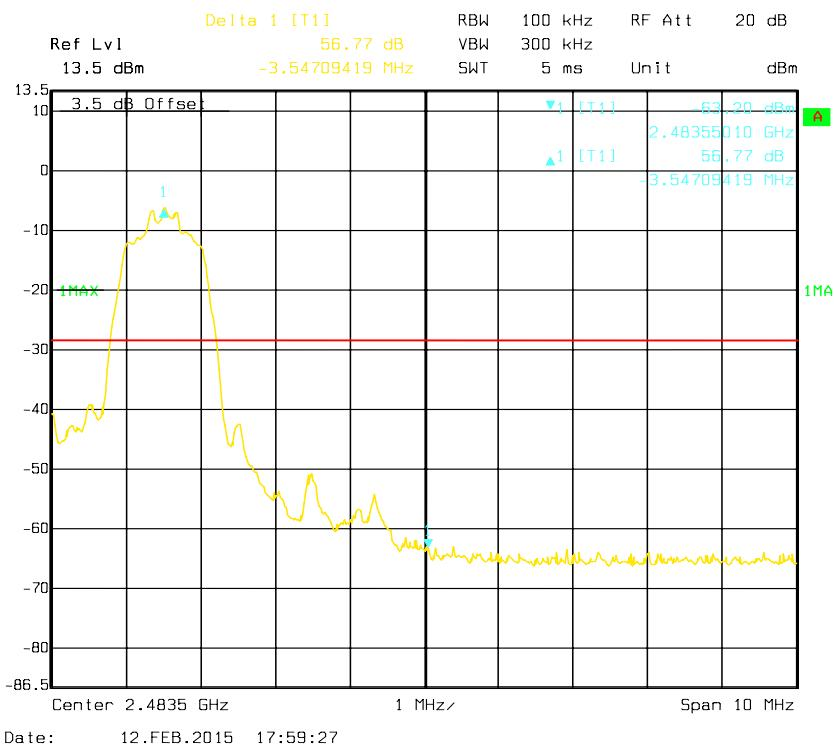
**EDR (8DPSK): Band Edge-Left Side**
