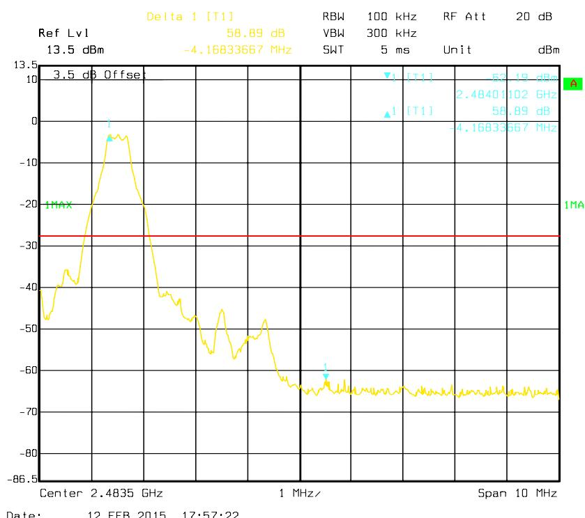
**EDR ( $\pi/4$ -DQPSK): Band Edge-Left Side**
