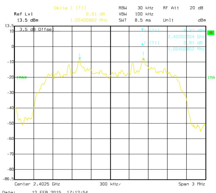
**EDR ( $\pi/4$ -DQPSK): Middle Channel**
