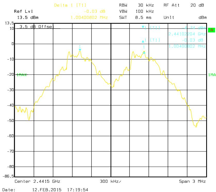
**BDR (GFSK): High Channel**
