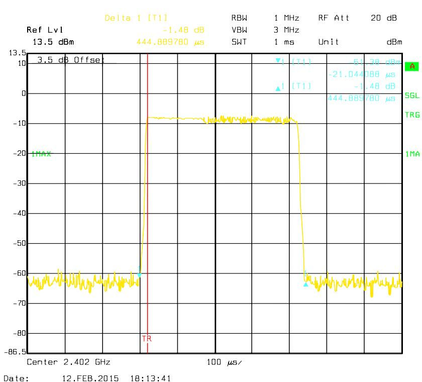
**Pulse time, Middle Channel, 2DH1**
