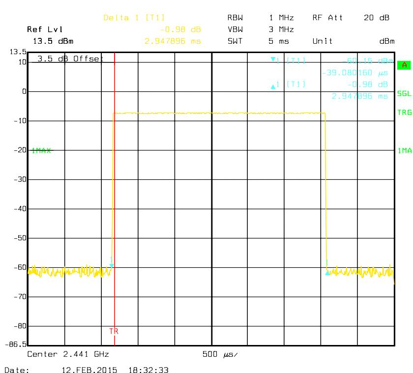
**Pulse time, High Channel, DH5**
