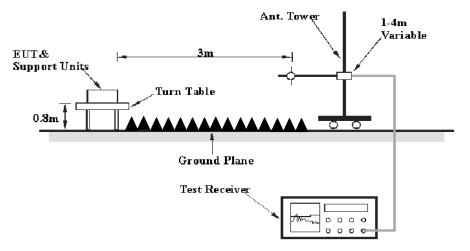
The radiated emission tests were performed in the 3 meters, using the setup accordance with the ANSI C63.4-2009. The specification used was the FCC 15.209 and FCC 15.247 limits.
