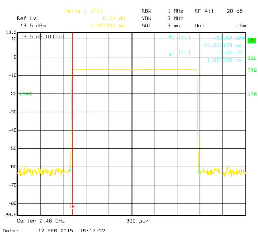
**Pulse time, Low Channel, DH5**
