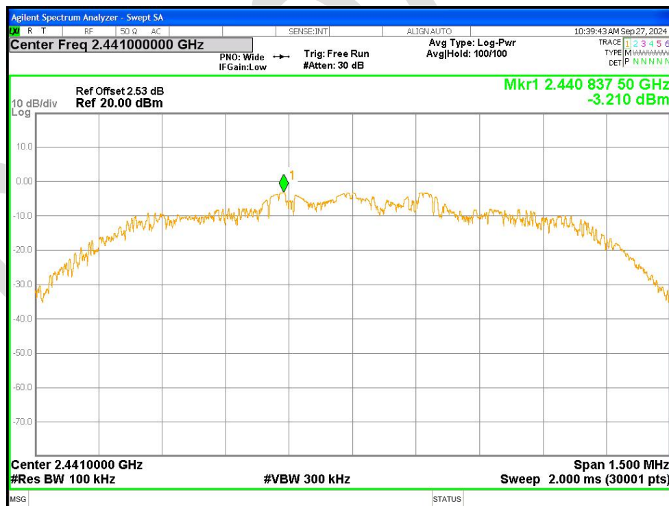
Tx. Spurious NVNT 3-DH1 2441MHz Ant1 Emission
